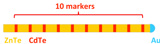
Figure 2.6: Growth recipe of sample M3194, with 10 CdTe sections used as markers. The experimental procedure is explained in section 2.1.3
