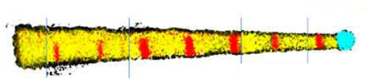
Figure 2.7: EDX image of a NW deposited on a holey carbon grid (composite of 5 higher resolution images). Colored areas are those where the Cd (red), Zn (yellow), Au (cyan) or O (black) signal exceeds an arbitrary threshold.
