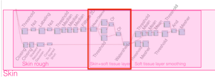
Figure 3.40: Footer scheme illustrating the part of the skin segmentation pipeline addressing skin and soft tissue layer segmentation (red rectangle).
