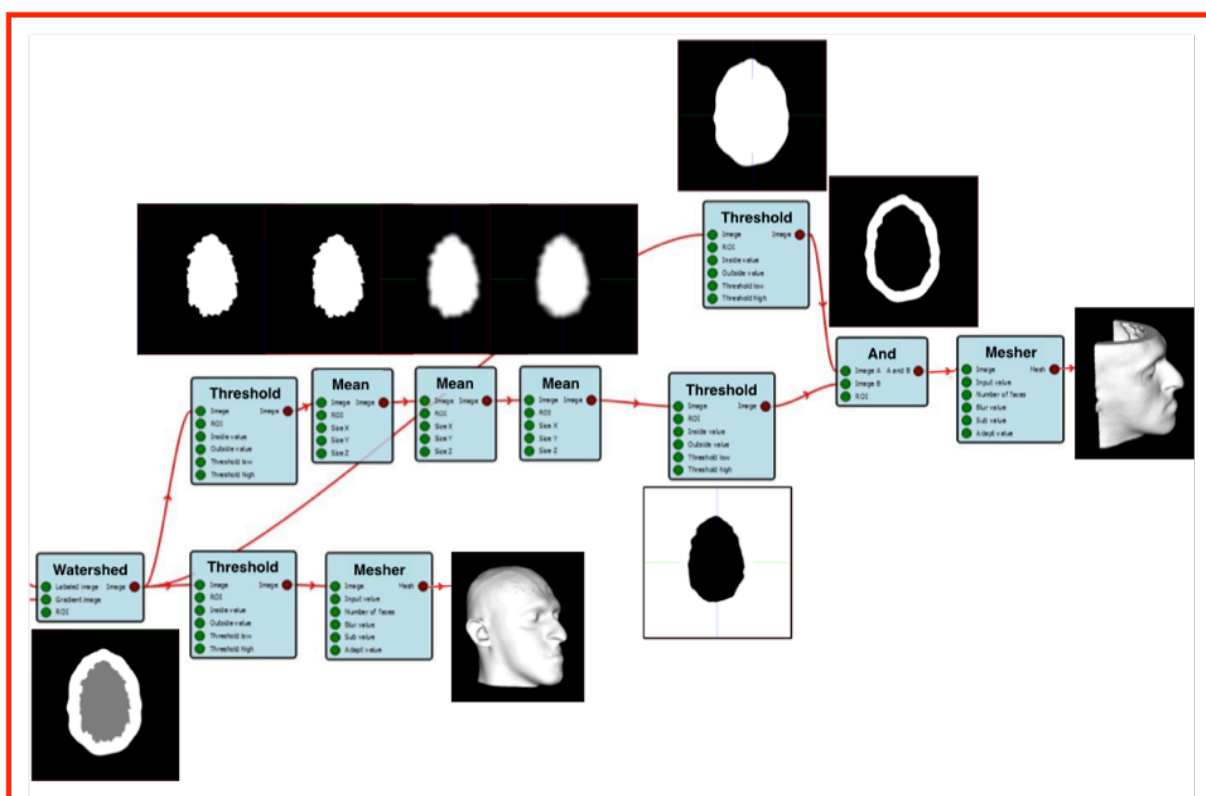
Figure 3.45: Detail of soft tissue layer smoothing pipeline. (Abstract from skin segmentation pipeline –Cf. Figure 3.32).
