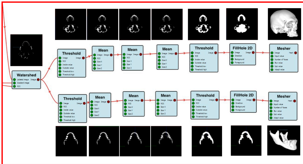
Figure 3.27: Detail of Bone image refinement segmentation pipeline (Abstract from global pipeline –Cf. Fig 3.12).
