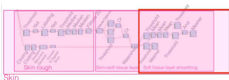
Figure 3.44: Footer scheme illustrating the part of the skin segmentation pipeline addressing skin outer surface extraction and soft tissue layer smoothing (red rectangle).
