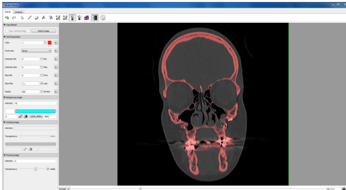
Figure 3.6: Propagation (in red) affecting the whole facial skeleton , since the skull and the mandible are linked due to contact between the upper and lower teeth, especially in this case where dental metal artifacts affect the image.
