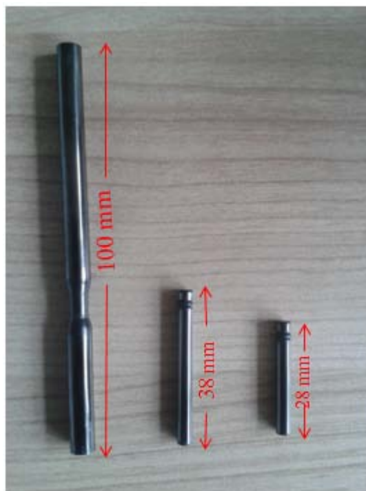
FIG. 2.11 - Photograph of a vitreous carbon cell used for absorption measurements X (absorption and fluorescence). The pistons are shown with length 38 mm and 28 mm.
