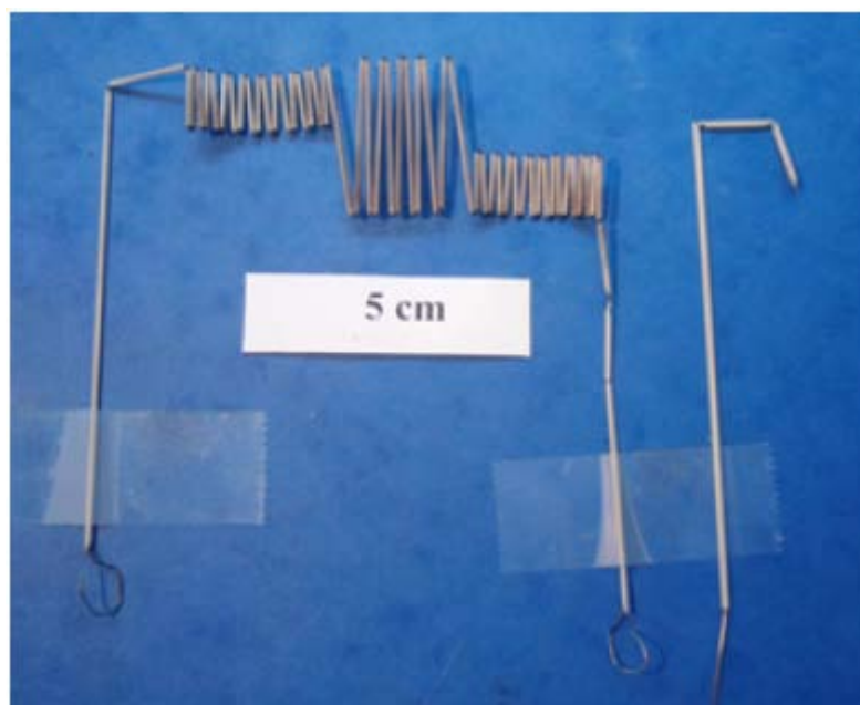
FIG. 2.10 - Photograph of an oven (left) and a thermocouple (right) used in our experiments.
