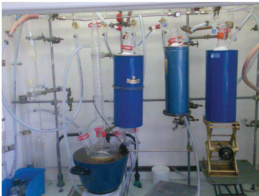
Figure III-1: Experimental procedure for borazine synthesis.
