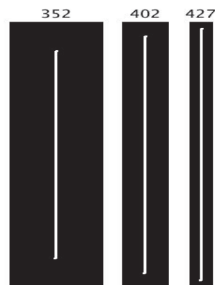
Fig. 1 Test image with three objects of identical maximum length (450 pixels) but of different thicknesses (100, 50 and 25 pixels from left to right); the skeletons (in white) are represented within the shapes of the original objects (in black), and their length (in pixels) is reported above each object, clearly illustrating the effect of object thickness on skeleton length.
