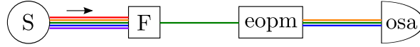
Figure 2.1: Experimental setup for phase modulation of classical light. A light beam emitted by source S is spectrally filtered by frequency filter F. The monochromatic light is sent through an electro-optic phase modulator EOPM, generating new frequencies, resolved with an optical spectrum analyzer OSA.
