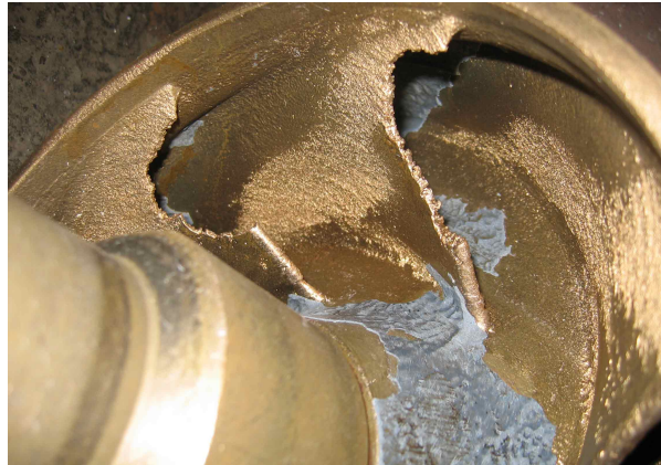
Figure 1.2: Damage of vane by cavitation.
