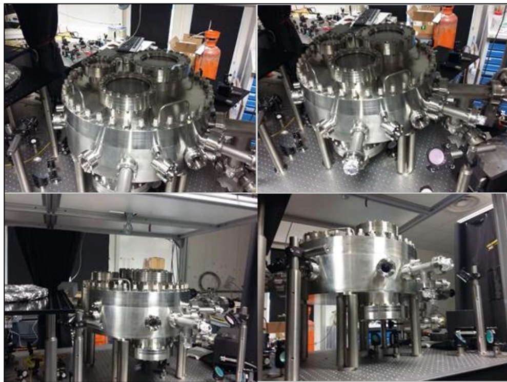
Figure 3.6: Different viewing angles of Ultra-High-Vacuum system (on laser table).
