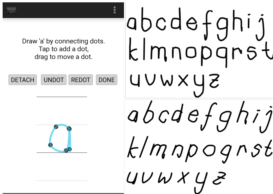
Figure 4.2: The font engine lets users to draw their own typeface by adding control points that are connected to a cardinal spline. Users can include several strokes by detaching the splines. On the right are two examples of static typefaces defined using the font engine: the baseline (top-right) and the variation (bottom-right).
