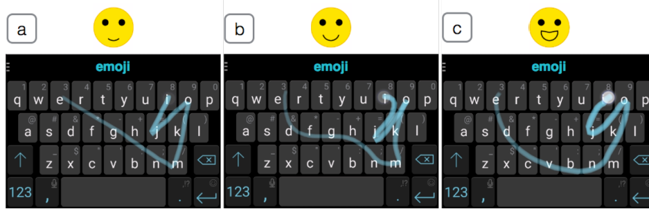
Figure 4.3: Manipulating the curviness and inflation in gestures with Expressive Keyboard will generate emoticons with subtle different of expression. a) A gesture with straight stroke segments generates a little smile; b) a curvy gesture generates a big smile; and c) a curvy, inflated gesture with wobbles at the end generates a laughing face.
