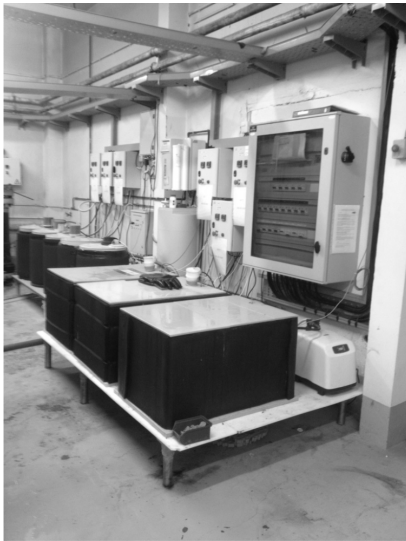
(a) Ageing tanks with continuously renewed natural seawater - IFREMER
