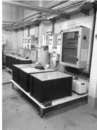
Figure 6.3: Ageing tanks with continuously renewed natural seawater - IFREMER
