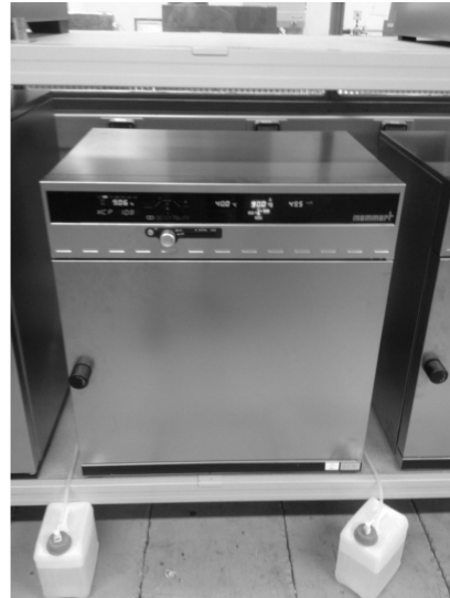
(b) Conditioning chamber for humid ageing at IFREMER
