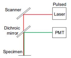
Figure IV.10: **2-Photon microscopy.** Two-photon microscopy setup: a pulsed near-IR laser is scanned over the tissue. The fluorescence emitted by the tissue is detected by a photomultiplier tube (PMT). Taken from [Grienberger and Konnerth, 2012].
