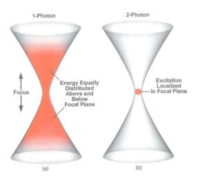
Figure IV.12: Localization of excitation in two-photon imaging. a) In one-photon imaging, the fluorescence occupies all the planes whereas in two-photon imaging (b), the fluorescence is constricted to a small volume around the focal plane. Taken from Murphy and Davidson, 2013].
