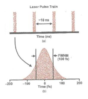
Figure IV.11: Pulsed IR laser used for two-photon imaging. A pulsed Titanium:sapphire laser with a) a pulse interval of  $\sim 10$ ns and b) pulse width of  $\sim 100$  fs. Taken from [Murphy and Davidson, 2013].
