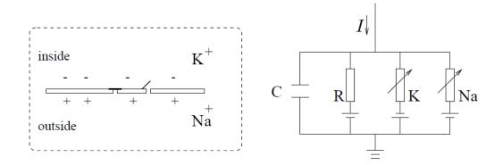
Figure I.2: A schematic diagram of the Hodgkin-Huxley Model. On the left is a description of the cell membrane, the ions inside and outside the cell and the ion channels. On the right is a circuit description of the neuron. The capacitance C represents the membrane. The active conductances represent the ion channels and the voltage sources represent the reversal potentials. I is the external current injected into the neuron. Taken from [Gerstner and Kistler, 2002].
