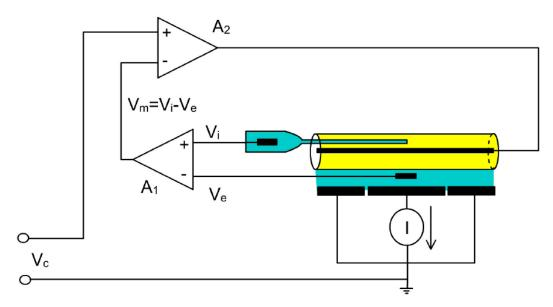
Figure I.1: Voltage patch clamp technique. The difference voltage,  $V_m$ , between the intracellular voltage  $V_i$  and the extracellular voltage  $V_e$  is maintained to be at  $V_c$ . This results in the injection of a current I, which is measured by an ammeter. Taken from http://nerve.bsd.uchicago.edu, Credits: F. Bezanilla.
