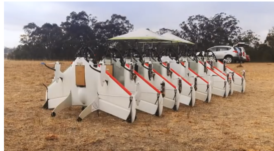
Figure 2.7 – Tail-sitter prototypes, as part of the Google's project Wing for delivery
