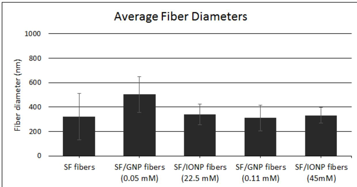
**Figure 2.12.** Average fiber diameters of electrospun SF-based fibers non-functionalized, functionalized with gold nanoparticles with a concentration of 0.05 mM or 0.11 mM, and functionalized with iron oxide nanoparticles with a concentration of 22.5 mM or 45 mM.
