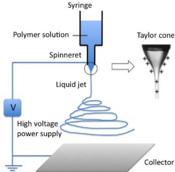
**Figure 19.** Setup for electrospinning simple, randomly deposited polymer nanofibers.
