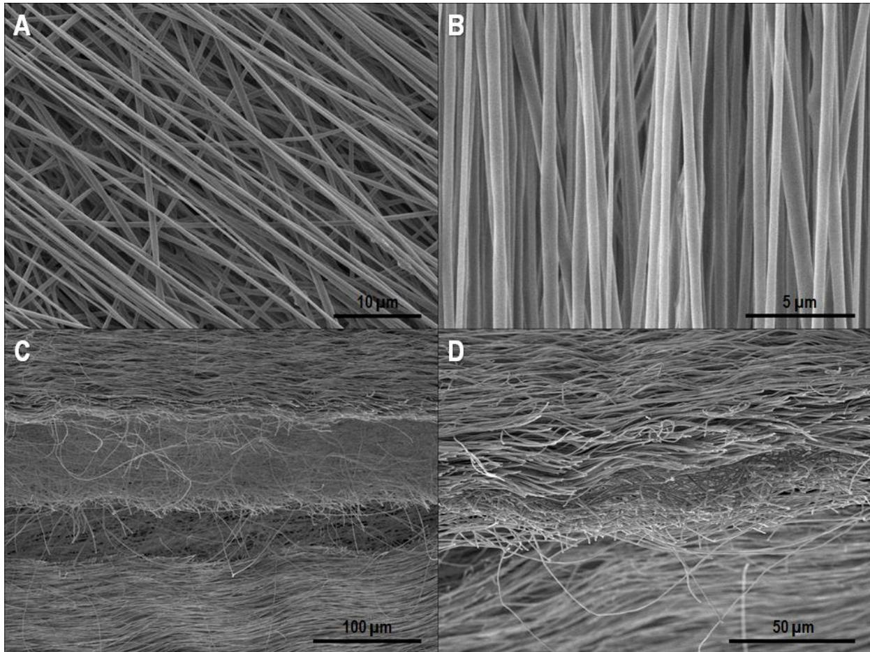
**Figure 1\*.** SEM images of (A) beginning of the final aligned layer deposited on center unaligned layer; (B) material's aligned surface layer; (C) & (D) cross sections of the tri-layered material after snap frozen in liquid nitrogen and sectioned longitudinally
