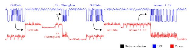
Figure 5.26 – Power consumption during a GetData command.
