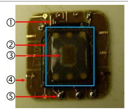
Figure 5.27 - ① Connection grid; ② Stolen card's module (outlined in blue); ③ Stolen card's chip; ④ FUN card module; ⑤ Weldings of connection wires.
