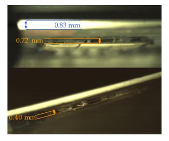
Figure 5.16 – Side-views of the forgery, showing that it is somewhat thicker than a standard card (0.83 mm). The extra thickness varies from 0.4 mm to 0.7 mm suggesting the existence of several components under the card module, besides the FUN card.
