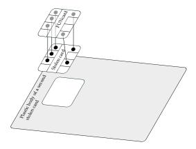
Figure 5.20 – Forgery structure suggested by Figure 5.19.
