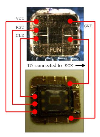
Figure 5.30 – Wiring diagram of the forgery.
