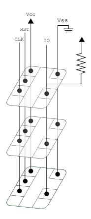
Figure 5.34 – Proposed low-cost HSM design based on SIM cards.
