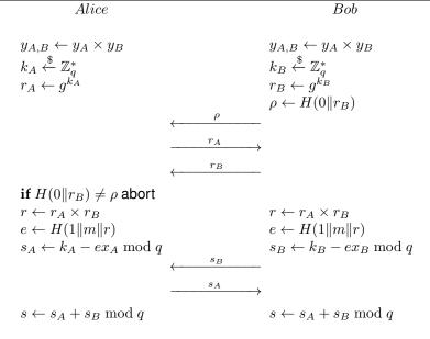
Figure 4.4 – Generating the Schnorr co-signature of message m.
