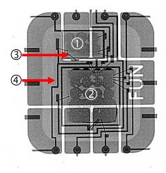
Figure 5.18 – FUN card X-ray analysis. ① External memory (AT24C64); ② Microcontroller (AT90S8515A); ③ Connection wires; ④ Connection grid.
