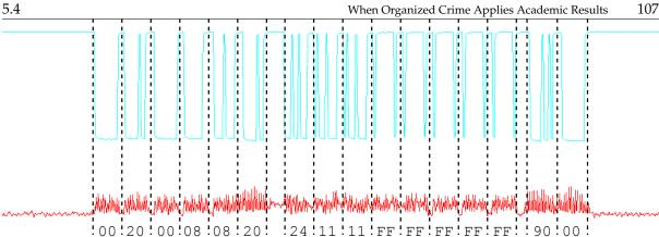
Figure 5.25 - Power trace of the forgery during the VerifyPIN command. Notice the absence of a re-transmission on the power trace before the returning of SW1 SW2.
