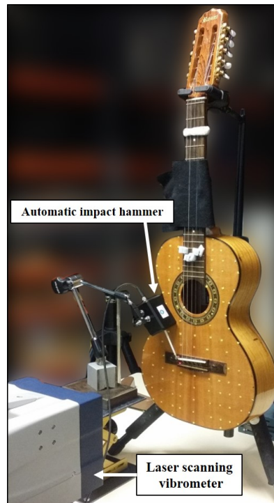
Figure 3.11: Setup composed by an automatic impact hammer and a laser scanning vibrometer used for measuring the vibration response on the front of the viola caipira .
