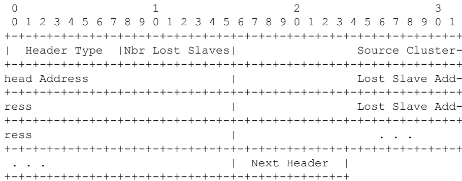
Figure 4.11: Format of the header for a Lost Slaves message (Textual representation).
