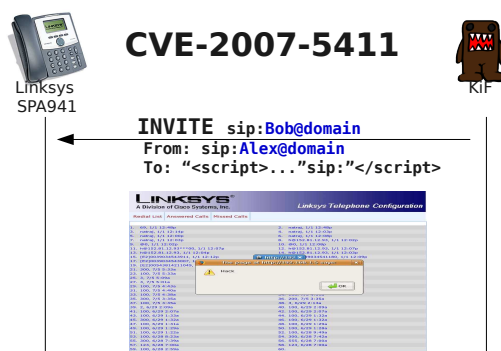
Figure 9.1: Linksys SPA-941 XSS attack
