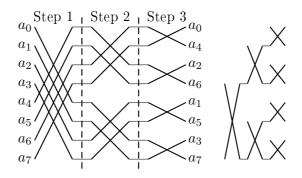
Figure 1.3: The FFT circuit of length 8 and a butterfly tree of depth 3.
