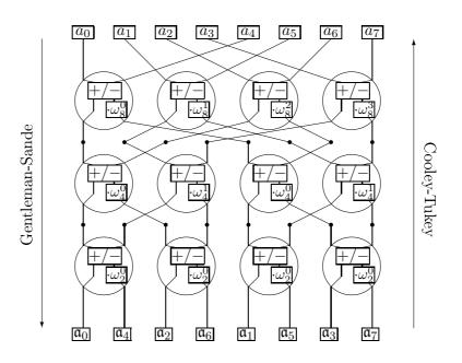
Figure 1.1: Data flow in a length-8 FFT. Here,  $\omega_n$  denotes an *n*-th primitive root of unity. Read from top to bottom, the diagram shows the data flow of the Gentleman-Sande algorithm with  $a_i$  as input coefficients and  $\mathfrak{a}_i$  as output. Read from bottom to top, it shows the data flow of the Cooley-Tukey algorithm, with  $\mathfrak{a}_i$  as input and  $a_i$  as output.
