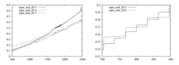
Figure 1.5: Time in milliseconds needed to multiply numbers modulo  $2^n + 1$  with an FFT of length  $2^k$  for k = 5, 6, 7. On the right, the zoom (with only k = 5, 6) illustrates that two curves can intersect several times.
