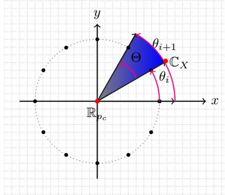
Figure B.1: Computing spatial relations using radial–line rotation. The rotation can be either clock-wise direction  $\ominus$  or  $\odot$ , however it must be fixed. In this illustration, we keep  $\odot$ . Radial–line rotation starts from the angle made by  $\mathbb{R}_{p_c}$  and  $\mathbb{C}_X$ .  $\mathbb{C}_X$  can be either  $\mathbb{C}_A$  or  $\mathbb{C}_B$ .
