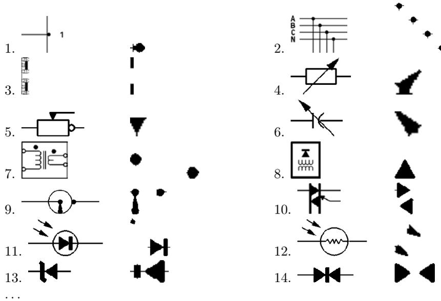
Figure 5.4: Symbols and their corresponding *thick* patterns. For visual understanding, *thick* patterns are zoomed out.
