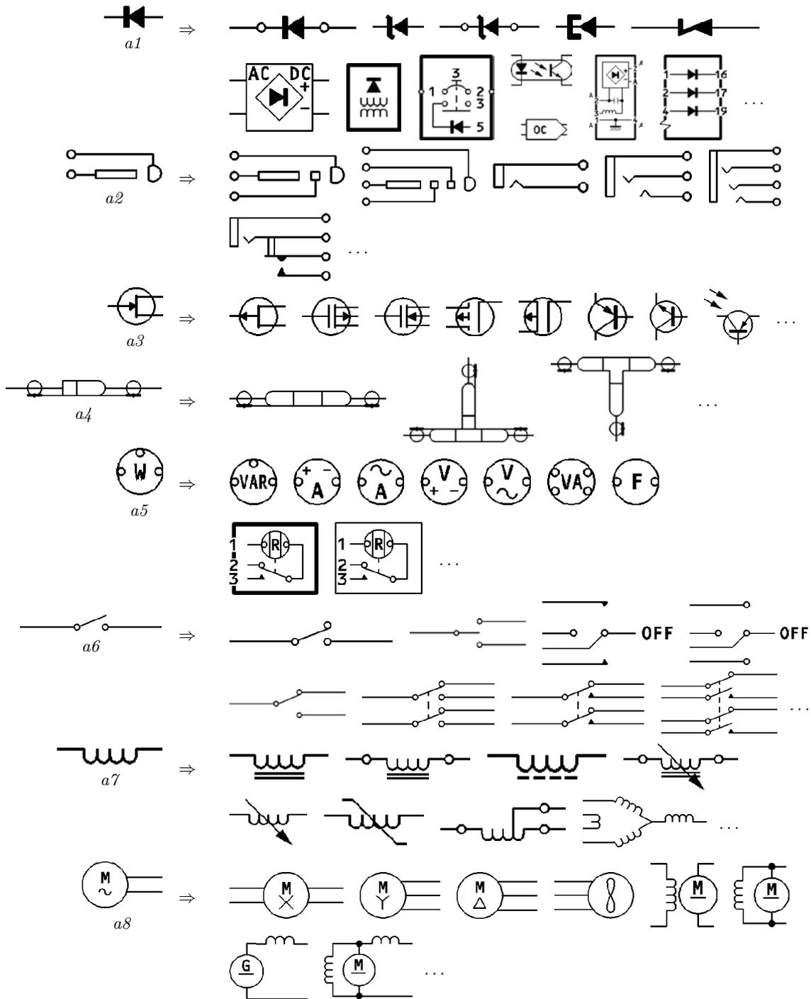
Figure 3.10: A sample of few electrical symbols and their similar sample images. For every test symbol:  $a_1$  to  $a_8$ , a few relevant symbols are enlisted based on human evaluation. It consists of both linear as well as symbols in the composite form.
