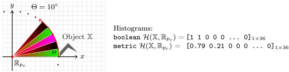
Figure 4.8: Relational histogram using radial line rotation.
