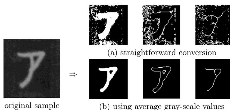
Figure 3.14: An example of binarisation sample from the ETL dataset.
