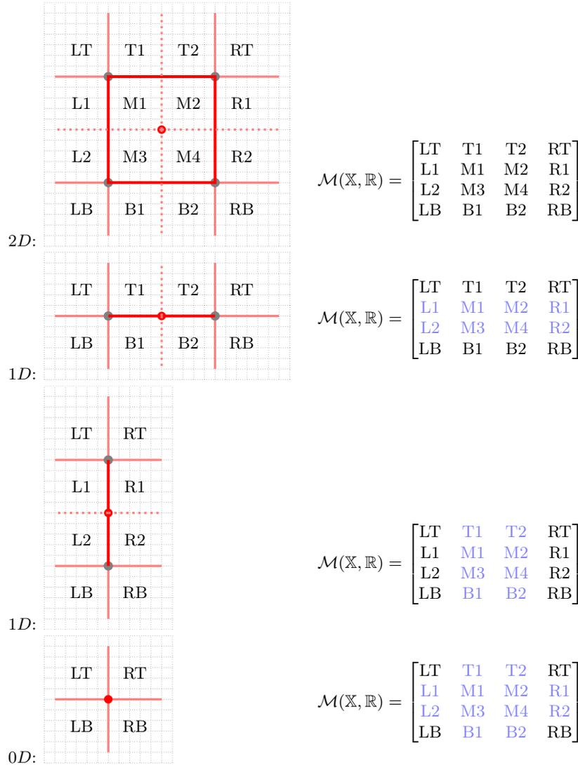
Figure 4.4: Projection models for all possible types of  $\mathbb{R}$  developed in Figure 4.3. Relational matrices are expressed following the corresponding models. The dimmed elements of the relational matrix  $\mathcal{M}$  refer to values equal to 0.
