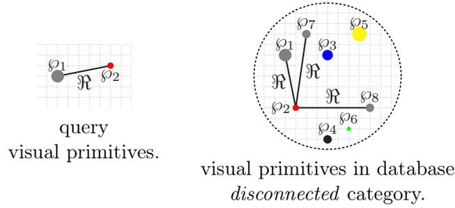
Figure 6.8: Relation matching example in a particular category: *disconnected*. Each item represents a visual primitive and colour represents its vocabulary type. Since query visual primitives are *disconnected*, the category is chosen accordingly. Moreover, vocabulary type information are taken into account for matching so that it avoids irrelevant matching.
