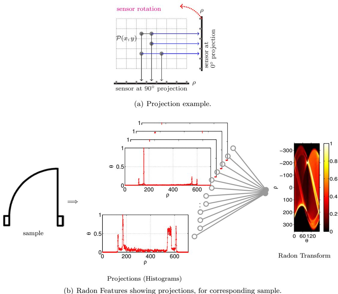
Figure 3.2: Radon transform – a complete illustration: (a) pattern projection using the Radon transform theory and (b) radon features for all possible projections over  $[0, \pi[$  and a complete radon transform i.e., a collection of all radon histograms or features.
