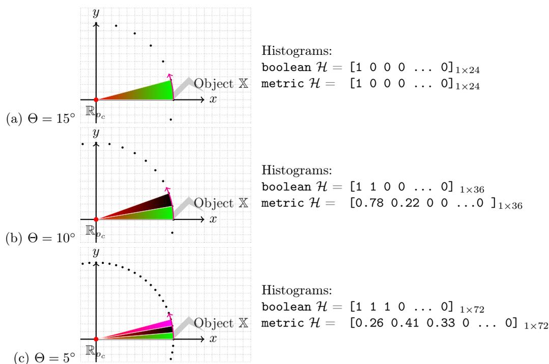
Figure 4.10: Different radial line resolutions effect precision. The smaller the  $\Theta$ , the higher the precision. In boolean signature, 1s represent the presence of  $\mathbb{X}$ . Metrical information provides the percentage.
