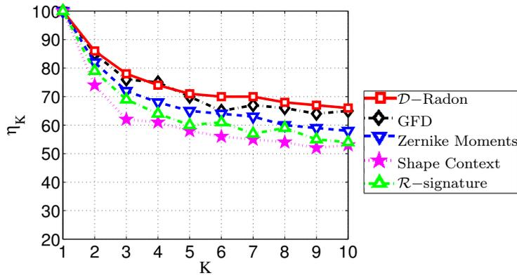
Figure 5.12: Average retrieval efficiency over requested list: 1 to 10 using global signal-based shape descriptors as vertex signature in our ARG framework.
