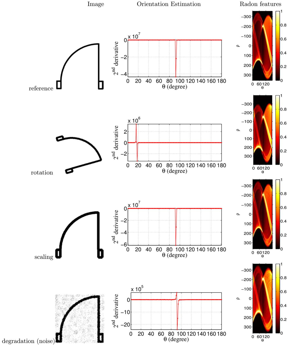
Figure 3.3: Images, their corresponding orientation estimation and the Radon features. Samples are taken from graphical symbol dataset [GREC, 2003]. Orientation angle  $\alpha$  has been estimated as follows:  $90^\circ$  for reference, scale and degradation images while  $17^\circ$  for rotation image.
