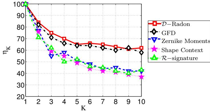
Figure 4.24: Average retrieval efficiency over requested list: 1 to 10 using global signal-based descriptors: Zernike moments, shape context, GFD,  $\mathcal{R}$ -signature and  $\mathcal{D}$ -Radon.
