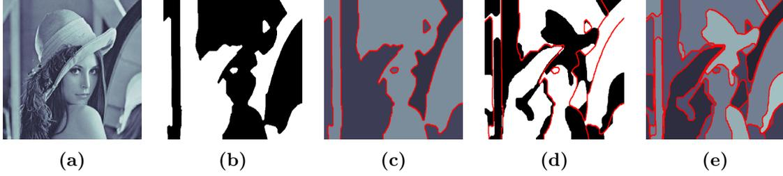
**Figure 4.3:** Two first iterations of cut pursuit for the ROF problem on the picture in (a). Images (b) and (d) represent the new cut at iterations 1 and 2 with  $B_\Pi$  and  $B_\Pi^c$  respectively in black and white, and (c) and (e) represent the partial solution in levels of gray, with the current set of contours  $S$  in red. The contours induced by the cut in (b) (resp. (d)) are superimposed on (c) (resp. (e)).
