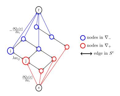
Figure 4.1: Directed graph for which finding a maximal flow is equivalent to solving (4.5). Neighboring nodes with different values of x in the original graph are linked by an undirected edge with capacity  $\lambda w_{ij}$ , nodes with non-negative gradient are linked to the source, and nodes with negative gradient to the sink with capacity  $|\nabla Q_S(x)|$ .
