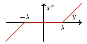
**Figure 2.1:** Set of solutions of the one-dimensional LASSO with square error fidelity  $\frac{1}{2}(x-y)^2$ . Red — represents the solution  $x^*$  for the different values of y.
