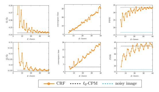
Figure 4.14: Behavior of the CRF algorithm for different number of quantization levels for the phantom (top) and the simulated data (bottom) averaged on 10 denoising experiments: (left) ratio between the energy Q at convergence and the energy at time 0, (middle) running time, (right) corresponding PSNRs. The two algorithms represented are  $\alpha$ -expansions (CRF) for a varying number of quantization levels and  $\ell_0$ -CPM.
