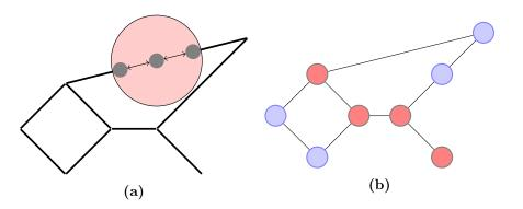
**Figure 6.1:** (a) Representation of a real graph with a zoom that shows that edges are actually a continuum of nodes linked by infinestimal unoriented edges. (b) The induced discrete graph associated with the junction nodes in red and the observed nodes in blue.
