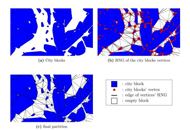
Figure A.7: Illustration of the computation of the polygonal partition. The relative neighborhood graph of the verices forming the city blocks 'a) is computed (b). Then the triangles joining the same blocks are merged (c).
