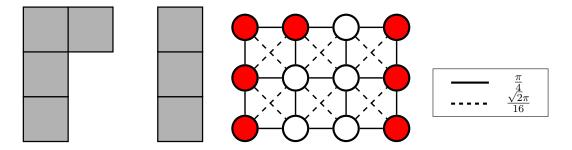
Figure A.2: Illustration of the conversion of raster data into a weighted graphs. Remark that the gaps are taken into account by adding empty cells.
