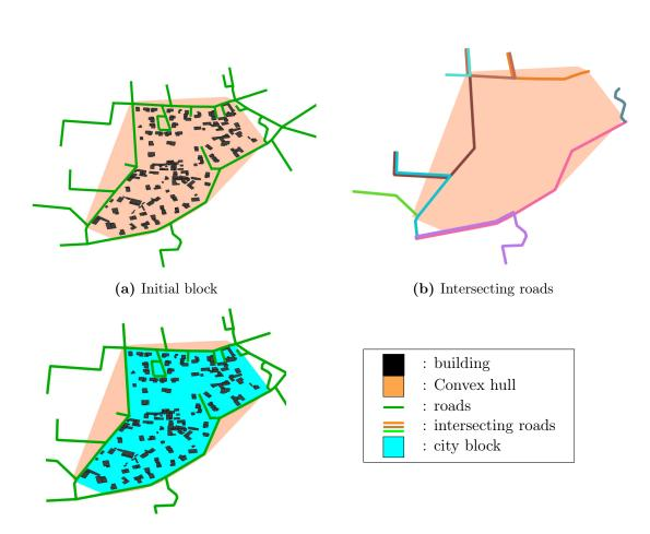
**Figure A.6:** Illustration of the computation of the shape of a city block. First the convex hull of all buildings is computed as well as the neighboring roads (a), then the *intersecting* roads are detected (b) and finally the city block is retrieved (c).
