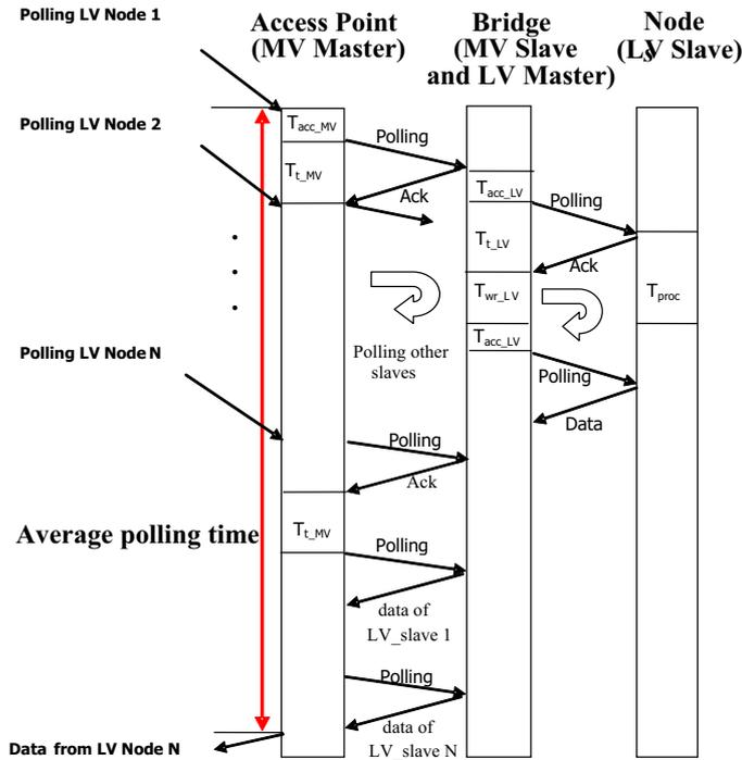
Figure 5.7: Schematic representation of average polling time at the Network Layer level in case of without cache in the slave
