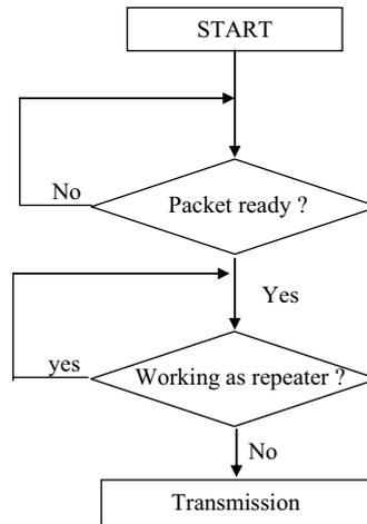
Figure 7.7: Block diagram of the ALOHA-SFN algorithm
