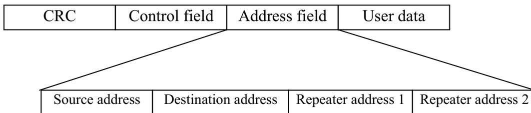
Figure 4.1: Structure of address field <sup>1</sup>
