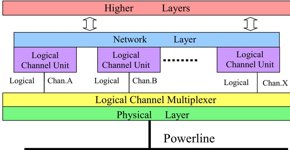
Figure 5.2: Layer concept with logical independent channels
