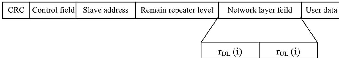
Figure 4.3: Structure of the SFN packet<sup>2</sup>
