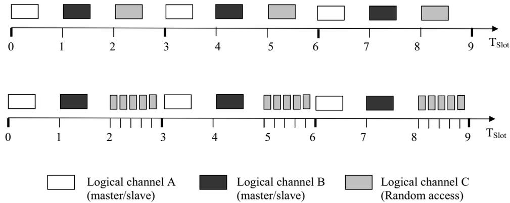
Figure 7.3: Illustration of the random access channel
