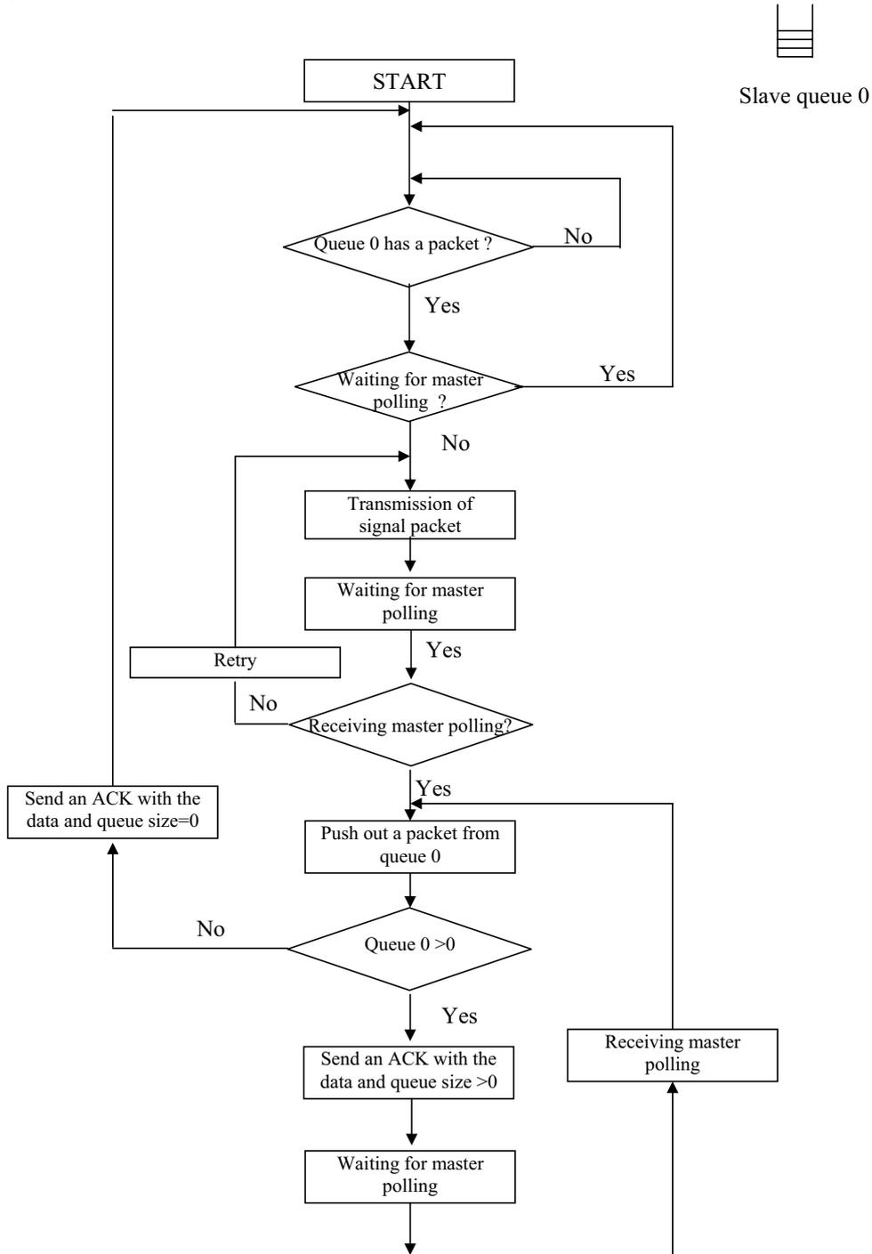
Figure 7.11: Block diagram of the slave transmission
