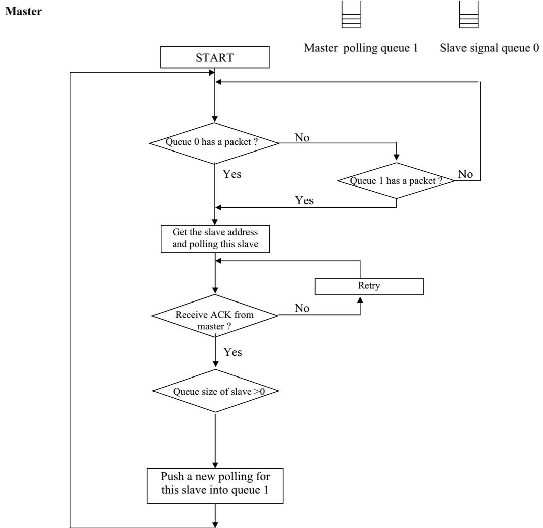
Figure 7.12: Block diagram of the master transmission
