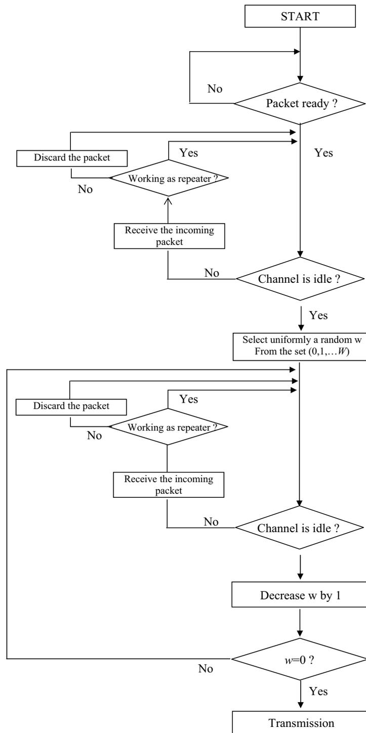
Figure 7.10: Block diagram of the predictive p-CSMA algorithm
