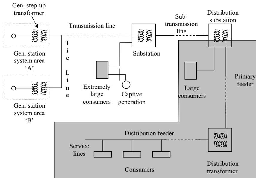
Figure 2.1: Schematic diagram of electric power distribution system
