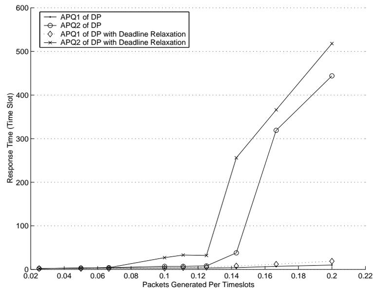
Figure 6.13: Response times of the aperiodic packets
