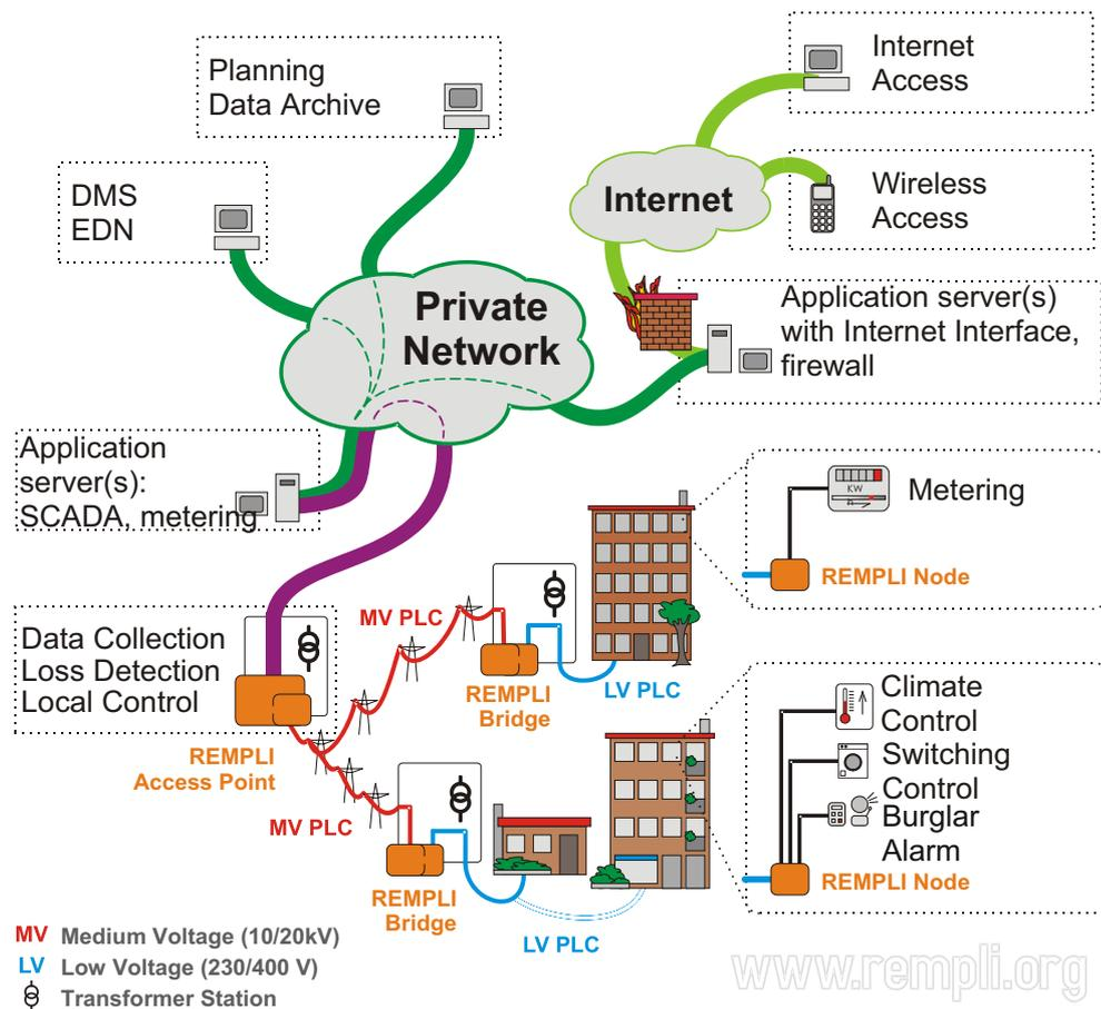
Figure 3.2: REMPLI system architecture, including the Private Network
