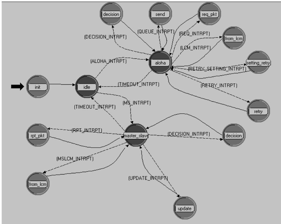
Figure B.22: Process model of network\_layer
