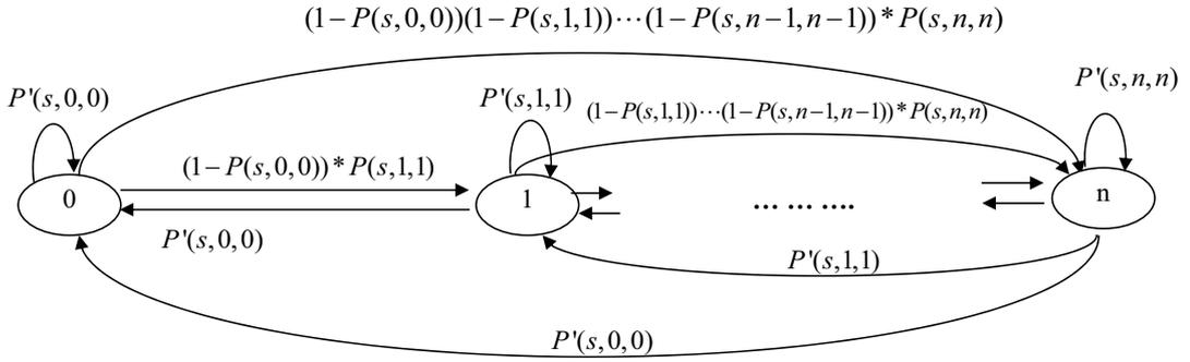
Figure 4.5: Markov chain model of repeater level
