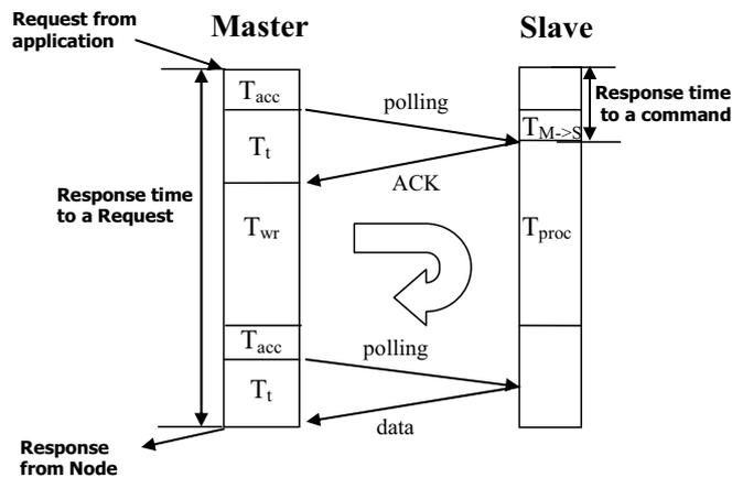
Figure 5.4: Schematic representation of application-to-application delay at the network layer level in an autonomous PLC network
