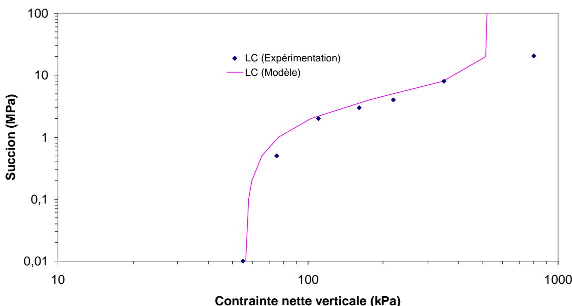
Figure II.46. Surfaces de charge (LC) initiale
