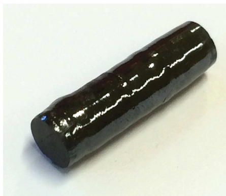
Figure 2.3: Sections of the as grown single crystal of SrFeO 2.5 .
