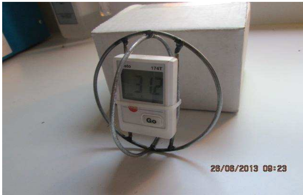
Figure.III.6. Support métallique des dataloggers.
