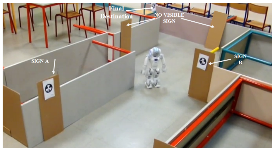
Figure 6.48: Test navigation environment. Only two signs from the sign sequence are placed in the environment.
