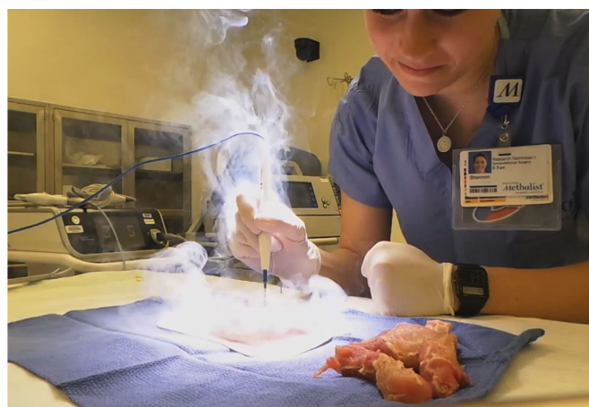
FIGURE 5.15: Smoke generated by the use of electrocautery instrument during our controlled tests on porc meat.
