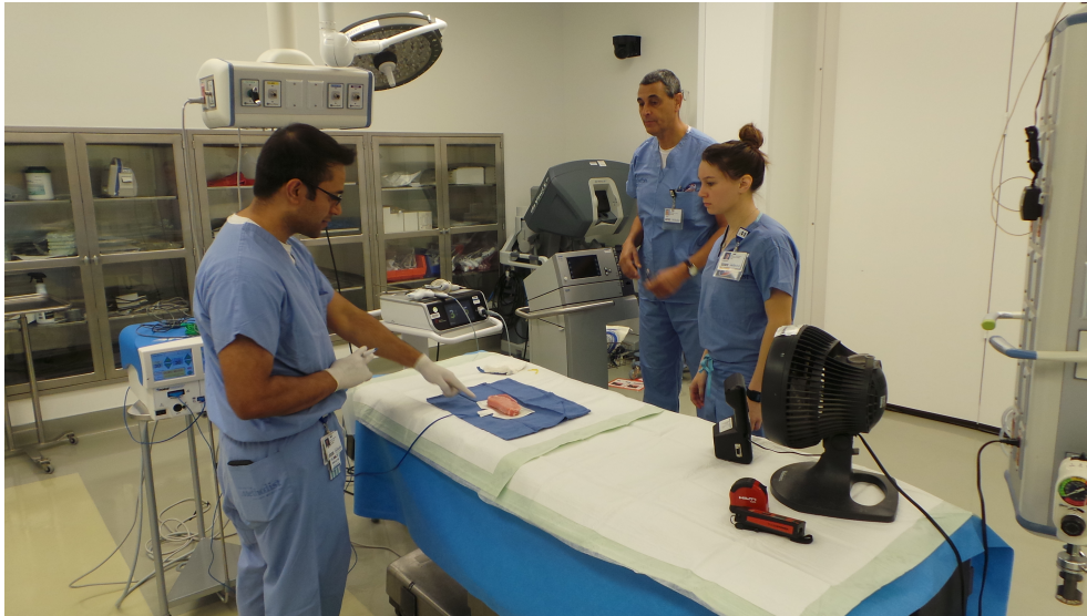
FIGURE 3.5: Settings of the test done on pieces of meat to understand the different smoke produced by common electrosurgical instruments.
