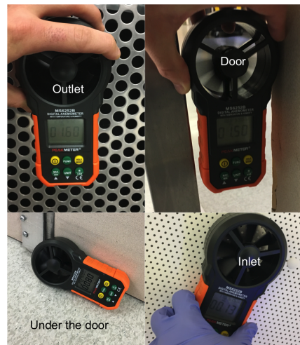
FIGURE 5.12: Measurements of velocities inside the studied OR with an anemometer.
