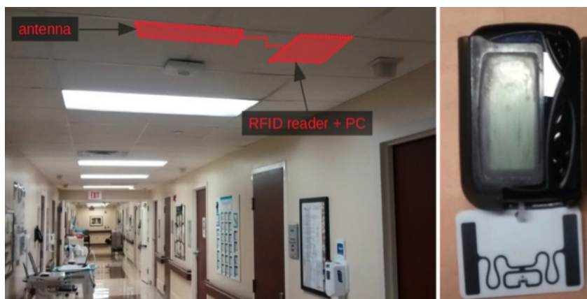
FIGURE 2.11: Installation of the RFID system at the entry of the preoperative area of the OR where the surgeon is supposed to go see his patient before a case. On the right, the RFID tag is placed on the pager of the surgeon.
