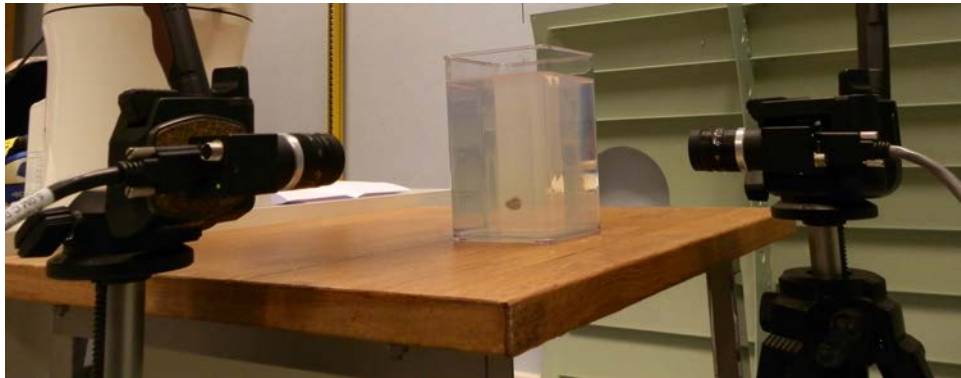
Figure 1.6: Picture of the stereo camera system and one gelatin phantom used for the experiments.
