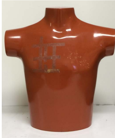
Figure 3.14. Anthropomorphic thorax phantom. The phantom is about 50 cm in height with a width and thickness of 28 cm and 19 cm, respectively, at the level of the heart.
