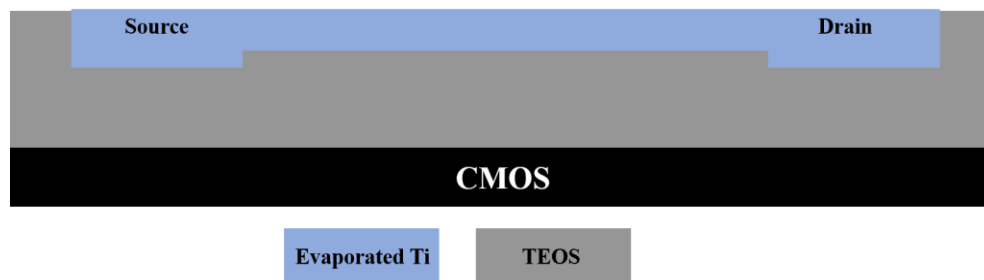
Figure 5.37 Schematic representation of cross-sectional structure of a Ti NW integrated in the TEOS layer on top of a CMOS substrate.
