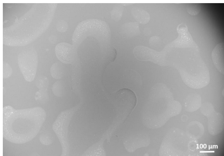
Figure 4.10 SEM image of CNT deposition by a single line pattern spray coating of a 0.1 mg/ml-concentrated MW-CNT dispersion in NMP at 40 mm/s of speed, 0.5 ml/min of flow rate and temperature of 70 °C.
