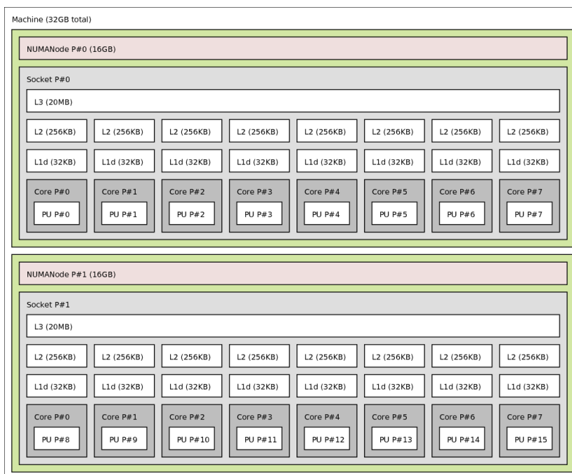
Figure 2.4 – Hwloc illustration on a dual-socket machine
