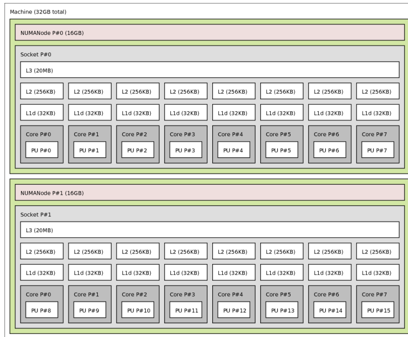
Figure 2.4 – Hwloc illustration on a dual-socket machine
