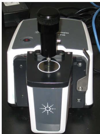
Figure 6. Cary 630 FTIR spectrometer from Agilent Technologies and laser signal input location.
