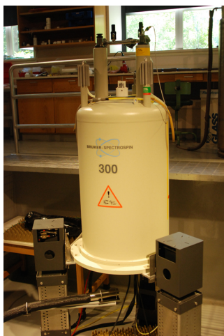
Figure 27. Bruker Avance 300 MHz (7 T) spectrometer.
