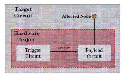
Fig. 2.2: Architecture of a Trojan inserted on a target circuit.
