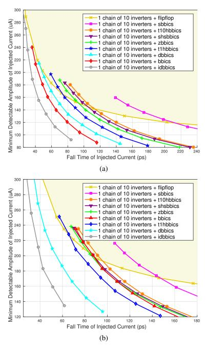
Fig. 4.13: Minimum injected currents  $I_{FaultN}$  (a) and  $I_{FaultP}$  (b) that are detectable by a BBICS architecture monitoring a chain of 10 inverters. Flip-flop's curves from Fig. 4.11 were redrawn here to indicate reference thresholds in which a single transient fault provokes a soft or delay error in the flip-flop.
