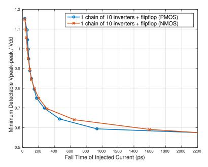
Fig. 4.10: Minimum peak-to-peak voltages (on node F and normalized to  $V_{DD}$ ) that are detectable by a flip-flop (Fig. 4.9) after the injection of single transient faults ( $I_{FaultP}$  or  $I_{FaultN}$ ) with fall times between 10 ps and 2200 ps; and a rise time on the order of 5 ps.
