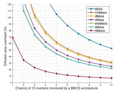
Fig. 4.15: Area overhead included by a BBICS architecture (a single sensor or one PMOS-BBICS and one NMOS-BBICS) that monitors a system with X chain(s) of 10 inverters (X between 1 and 10).
