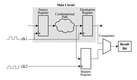
Fig. 2.10: Delay characterization with negative-skewed shadow registers [80].
