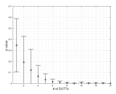
Fig. 5.6: Progress of p-value (with accuracy of  $\pm \sigma$ ) in function of the number of DUTTs.
