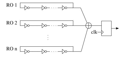
Fig. 3.2: The RO-based TRNG design.
