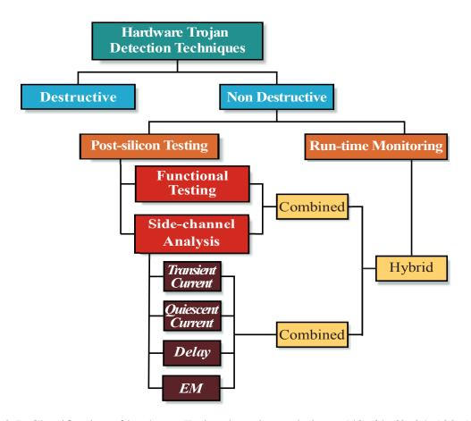
Fig. 2.7: Classification of hardware Trojan detection techniques [48, 64, 69, 94, 130, 132].
