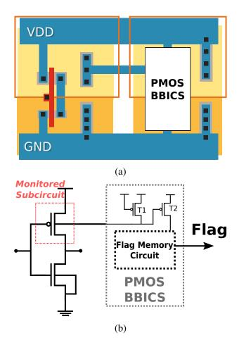
Fig. 5.2: Layout of an inverter monitored by a PMOS BBICS (a) and its schematic view (b).
