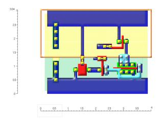
Fig. 4.8: Layout of the new dynamic NMOS-BBICS cell on CMOS 65 nm technology. The divisions of the axis are in  $\mu m$ . The area of the proposed cell is comparable to the sum of three technology NAND cells with minimum drive capabilities. The layout design of the PMOS-BBICS cell, which is not illustrated here, is complementary to this figure.
