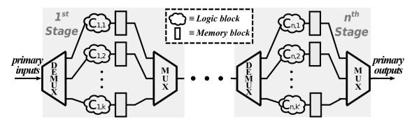
Fig. 6.4: Diagram of a pipelined system with *n* stages.
