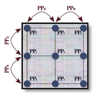
Fig. 2.9: Chip partition approach based on the measurement of multiple power supply pins for Trojan isolation [114, 115].
