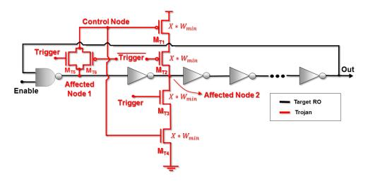
Fig. 3.5: Transmission-gate Trojan isolable by high impedance from the RO.
