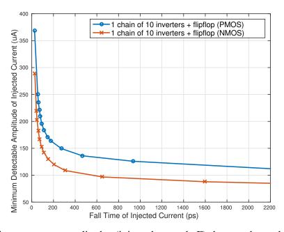
Fig. 4.11: Minimum current amplitudes (injected on node F) that are detectable by a flip-flop (Fig. 4.9). The related injected currents, in function of different fall times (horizontal axis), create the peak-to-peak voltages illustrated in Fig. 4.10.
