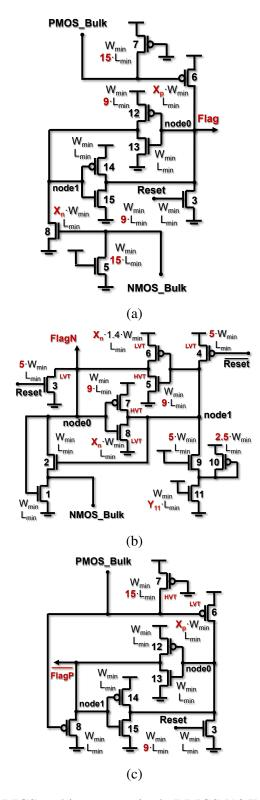
Fig. 4.3: State-of-the-art BBICS architectures: single BBICS [125] (a), NMOS-BBICS of Neto et al. [102] (b), PMOS-BBICS of Zhang et al. [150] (c).  $W_{min}$  represents the minimum diffusion width of the transistors,  $L_{min}$  is the minimum channel length, and  $X_n$  and  $X_p$  are design factors used for calibrating the sensitivity of the sensor in detecting transient faults.
