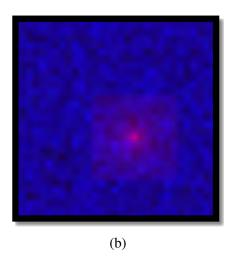
Fig. 2.11: EM emission maps generated considering a Trojan free DUTT (a); and a Trojan-infected DUTT (b). For each pixel, blue shades represents low difference between EM emission from golden device and DUTT, and red shades denotes considerable discrepancies [14, 129].
