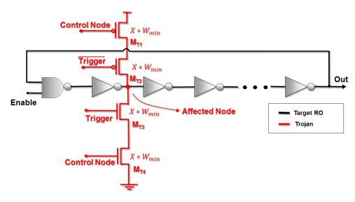
Fig. 3.4: Double-switch Trojan isolable by high impedance from the RO.
