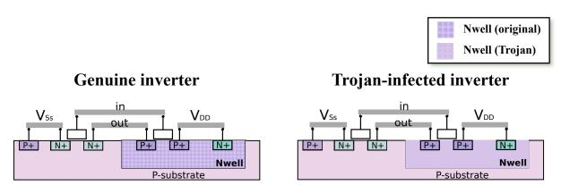
Fig. 2.6: Layout of an inverter with the dopant Trojan presented in [72].
