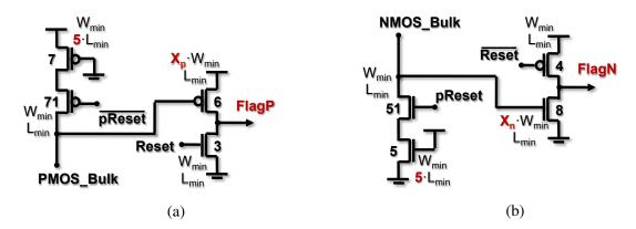
Fig. 4.6: New dynamic BBICS architectures (a) and (b) proposed in this chapter for detecting transient faults in pull-up and pull-down CMOS networks. The bulks of the PMOS and NMOS transistors under monitoring are biased, respectively, by the voltages on PMOS\_Bulk and NMOS\_Bulk nodes, rather than the voltages on the power rails  $V_{DD}$  and GND.  $W_{min}$ ,  $L_{min}$ ,  $X_n$ , and  $X_p$  are defined in captions of Fig. 4.3.
