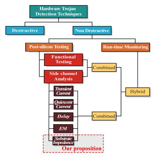
Fig. 5.1: Classification of hardware Trojan detection techniques [48, 64, 69, 94, 130, 132] with a new category of side-channel analysis: the substrate impedance.
