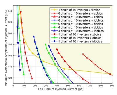
Fig. 4.14: Minimum injected currents I<sub>FaultP</sub> that are detectable by a PMOS-BBICS architecture monitoring either 1, 4, or 6 chains of 10 inverters.
