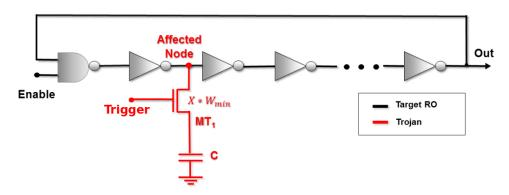
Fig. 3.3: Capacitor Trojan isolable by high impedance from the RO.
