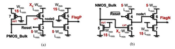
Fig. 4.5: Dynamic BBICS architectures (a) and (b) of Simionovski and Wirth [126] for monitoring transient faults, respectively, in pull-up and pull-down CMOS networks.  $W_{min}$ ,  $L_{min}$ ,  $X_n$ , and  $X_p$  are defined in captions of Fig. 4.3.
