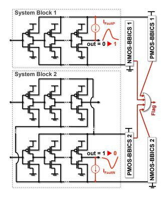
Fig. 4.2: Basic illustrations of BBICS monitoring two system blocks.  $I_{FaultP}$  and  $I_{FaultN}$  are current sources acting as external perturbations that produce abnormal current effects on the circuit defined as transient faults.
