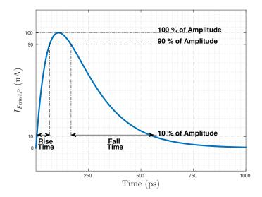
Fig. 4.1: Typical double-exponential profile of a transient fault, which is defined as a transient current generated on the circuit by a external perturbation such as radiation sources or laser beams.
