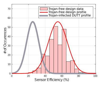
Fig. 5.5: Histogram of the sensor efficiency for Trojan-free design surrounded by its profile curve and another one of a Trojan-infected DUTT.
