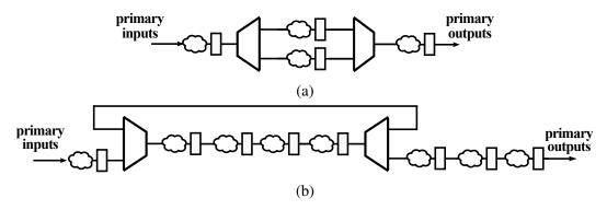
Fig. 6.5: Representation of the circuit pipeline stages from the ALU proposed by [37] (a) and a typical AES [7] (b).
