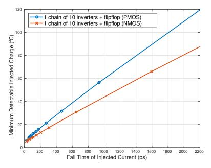
Fig. 4.12: Minimum charges (injected on node F) that are detectable by a flip-flop (Fig. 4.9). The related injected currents, in function of different fall times (horizontal axis), create the peak-to-peak voltages illustrated in Fig. 4.10.
