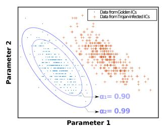
Fig. 2.8: Space of parameters generated by the data obtained from golden devices – error ellipses with difference significance levels  $\alpha_1=0.90$  and  $\alpha_2=0.99$  surround it –, and from Trojan-infected DUTTs.
