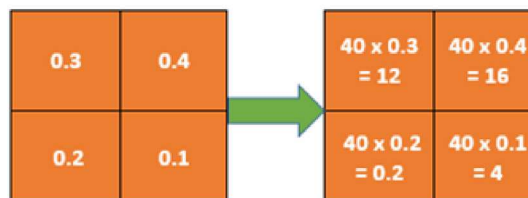
Fig. 3. Sub-pixel AMSR-E data extraction using probability distribution.
