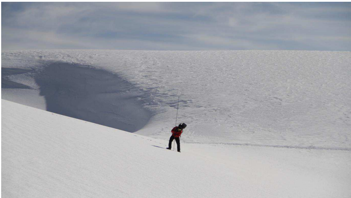
Measuring snow height (HS) and snow density. Cedars (2870 m), 6 Mar 2016. Photograph by C. Abou Chakra
