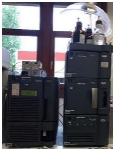
Figure 21 : Acquity UPLC H-Class (Waters) couplé à un triple quadrupôle (Acquity TQ Detector, Waters)
