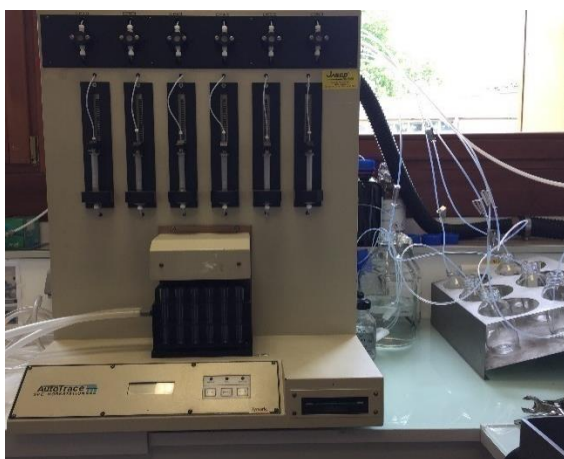
Figure 23 : AutoTrace SPE Workstation, Zymark
