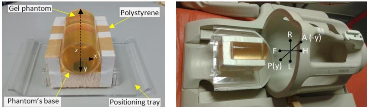
Figure 3.8. Gel phantom analysis by MRI with the head coil: (left) irradiated gel phantom on the positioning Plexiglas tray and the polystyrene blocks; (right) placement of the phantom and positioning tray inside the head coil where the system of coordinates indicates the final position for reading.
