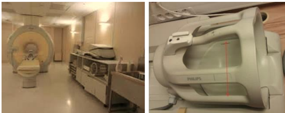
Figure 3.7. (Left) the imaging room of the SHFJ with the MRI Philips imager inside and (right) the head coil.
