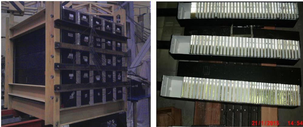
FIGURE 6.16: View of the hadron calorimeter setup (left) and of the scintillators in each module (right).
