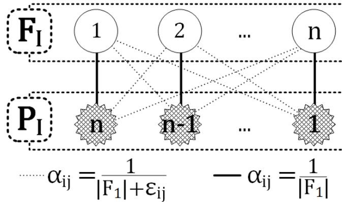
Figure 6.14 Intersection points renumbering and capture rates assignment
