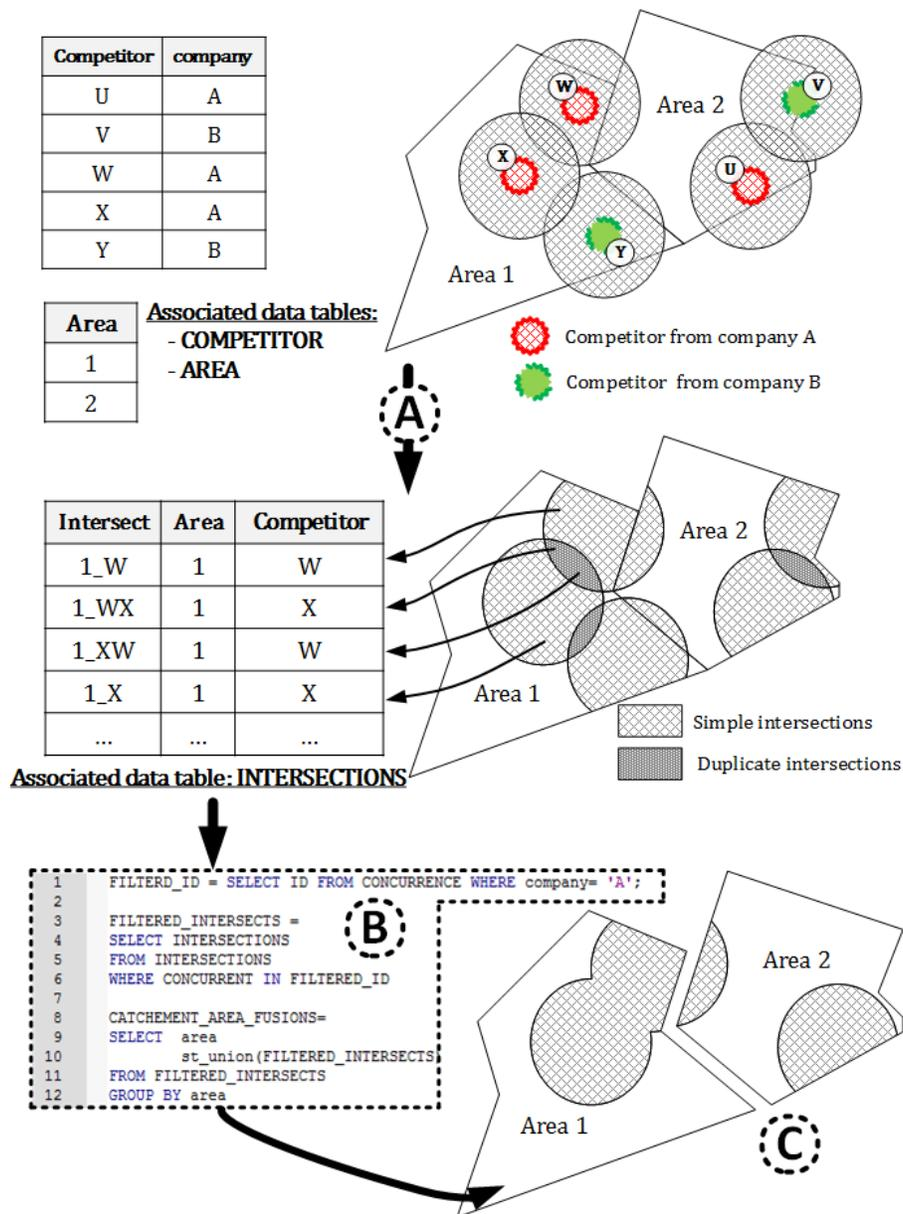
Computations of intersections in those layers are only processed when a new element is added to a Source or a Target Layer or when a new Source Layer or a new Target Layer is imported into the database.
