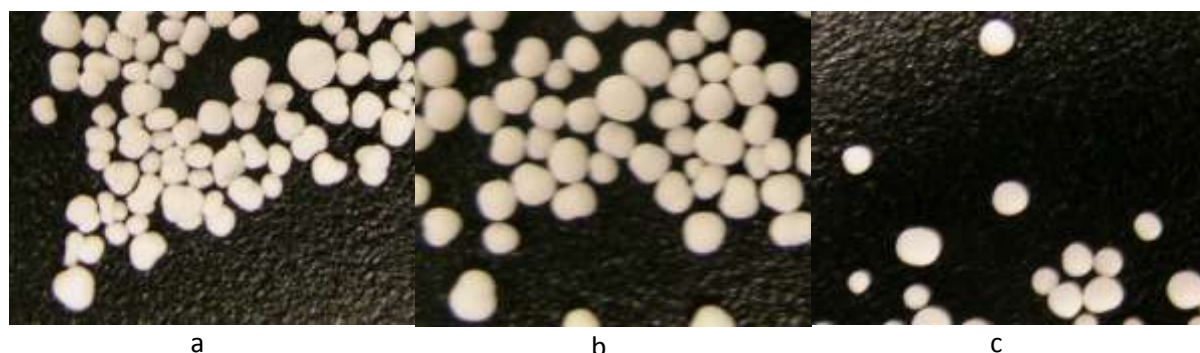
Figure 3.4. Light microscopy images of pellets with different spheronization times: a. 2 minutes, b. 6 minutes, c. 10 minutes
