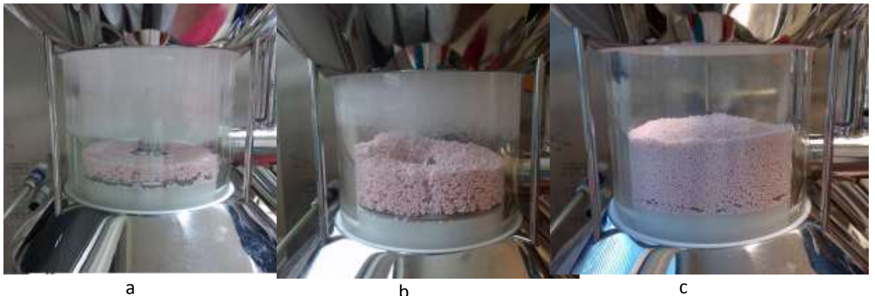
Figure 5.9. Depositing of coating material on the walls of the partition with three different inventories 15 % (a), 30% (b), 50% (c) of the maximum capacity in the product container IPC1.
