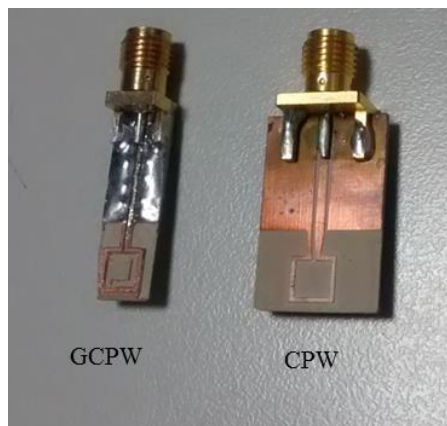
Figure 3-22 Fabricated probes with CPW and GCPW transmission lines
