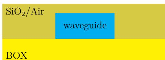
Figure 5.1: Waveguides section geometry.
