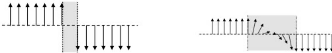
Figure 1.4: Scheme of magnetization reversal according to the width of the domain wall (the reversal is abrupt in a very thin domain wall and continuous in a large domain wall). A narrow domain wall has a high exchange energy (**left**) and a wide domain wall has a high anisotropy energy (**right**).
