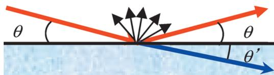
Figure 3.3: Reflection and refraction of X-Rays on material surface.
