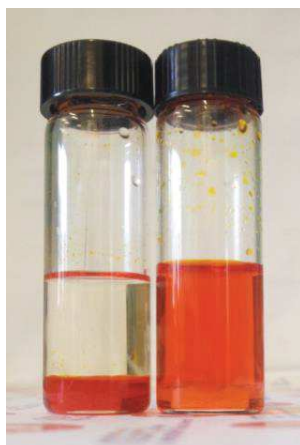
Figure 5. Biphasic water/IL solutions after contacting the MO containing water phase with C 6 Gua NTf 2 (left) and C 4 mim NTf 2 (right)
