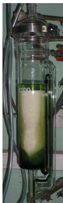
Figure 4.6 Picture of the 2L Soxhlet apparatus used for the extraction of chlorophyll a .
