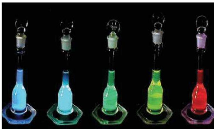
Figure 3.16 Picture of the PPE-Ar-SO 3 - fluorescence in methanol under UV illumination (from the left to the right: Ph, Py, Th, EDOT, BTD). 30
