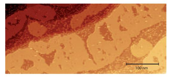
FIGURE 3.15: STM image at large scale of the flat islands that appear after 15 minutes at  $300^{\circ}$ C. The tilting of the image is due to the drift correction, as explained in the experimental section. V=-3.9 V; I=300 pA.
