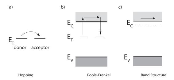
FIGURE 1.5: The different conduction models: a)hopping; b)Poole-Frenkel trap and release; c)bands. Image adapted from ref. [131],  $E_V$  is the valence band energy,  $E_T$  is the energy of the trap states,  $E_C$  is the conduction band energy.
