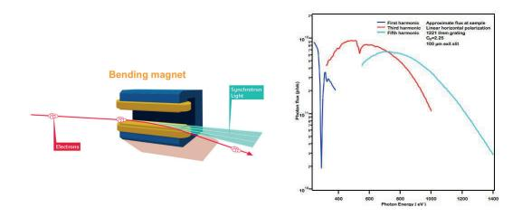
FIGURE 2.1: Working principle of a bending magnet (left); Emission spectrum of the bending magnet at the I1011 at Maxlab (right).
