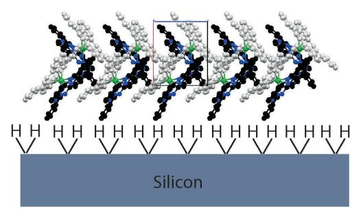
FIGURE 3.4: Depiction of the molecular stacking of LuPc<sub>2</sub> on H terminated Si(100).
