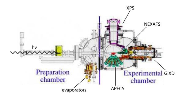
FIGURE 2.5: Image of the geometry at beamline Aloisa.
