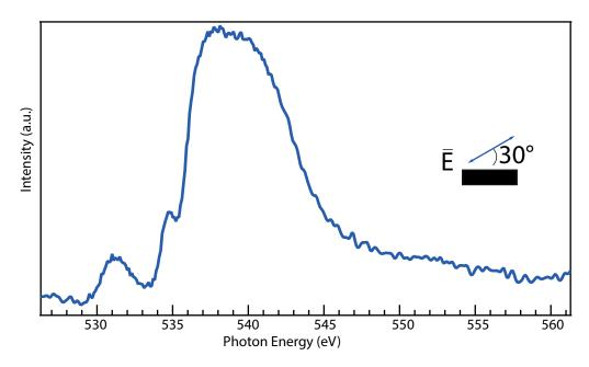
FIGURE 4.11: NEXAFS spectrum of LuPc $_2$ /Au(111) at the O K-edge taken after exposition to 90000 L O $_2$  at 88 K.
