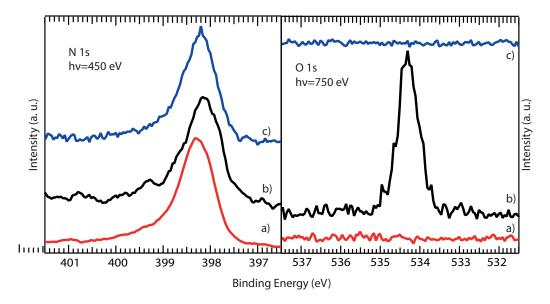
FIGURE 4.12: XPS spectra of  $LuPc_2/Au(111)$  exposed to water. The N 1s (right) and O 1s (right) before (a), are shown during and after the  $H_2O$  exposure.
