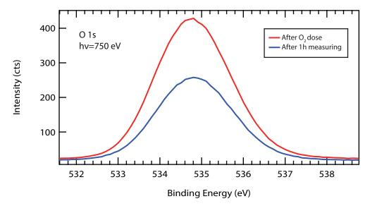
FIGURE A.2: XPS spectrum of a  $\pm 3$  nm thick LuPc<sub>2</sub> thin film deposited on Au(111) after measuring for half an hour (a) and on a fresh spot (b).
