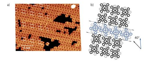
FIGURE 3.23: a) STM image showing different domains V=-2.6 V, I=700 pA; b) model of the two different domains as deduced from the STM image.
