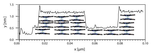
FIGURE 3.16: top: STM image of an island. V=-2.6 V; I=300 pA; bottom: profile obtained over the line shown on the STM image, with a depiction of the molecular stacking (the horizontal axis is not on scale).
