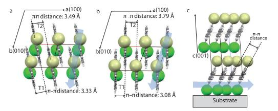
FIGURE 1.6: Molecular packing structure of TIPS-pentacene thin films prepared under different conditions: a) thermal evaporation; b)deposited by spin coating; c) same as b) but along the cofacial axis.
