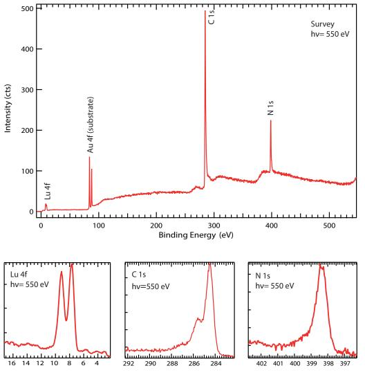
FIGURE 4.1: XPS spectra of LuPc<sub>2</sub>  $\sim$ 1 nm deposited on Au(111). a) Survey; b) Lu 4f; c) C 1s; d) N 1s.
