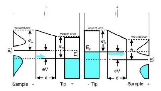
FIGURE 2.15: Changes in tip-sample system energy and tunnelling conditions as the bias polarity is inverted.
