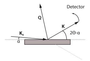
$\label{figure 2.21: Schematic depiction of GIXD geometry.}$
