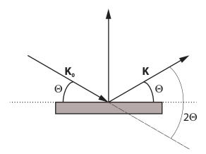
FIGURE 2.18: Schematic representation of a  $\theta/2\theta$  experimental setup.
