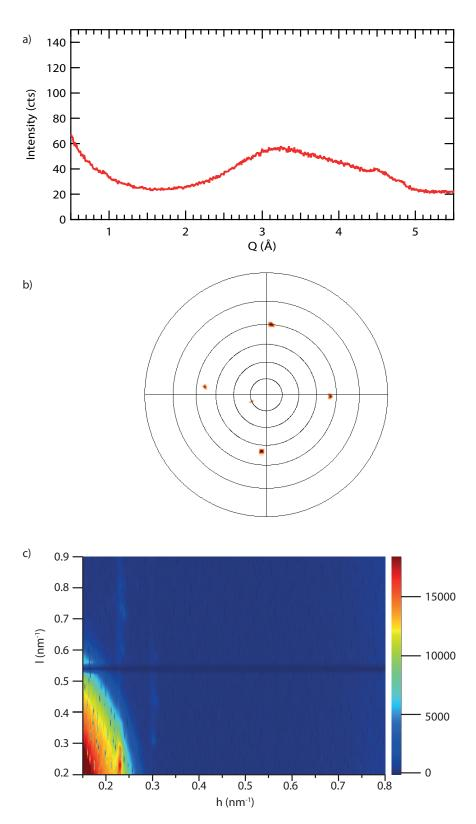
FIGURE 2.19: Example of the different X-ray diffraction techniques used in this work: a)  $\theta/2\theta$  scan of LuPc<sub>2</sub> on H terminated Si(100); b)pole figure on the Si(111) peaks of LuPc<sub>2</sub> on H terminated Si(100); c)out of plane map of LuPc<sub>2</sub> over Au(111).
