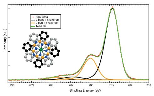
FIGURE 4.3: Resolution of the single spectral components of XPS spectrum of the C 1s peak of a LuPc<sub>2</sub> thin film ( $\sim$ 1 nm) deposited on Au(111).
