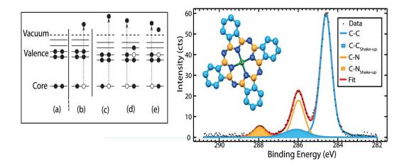
FIGURE 2.10: Left: schematic of the different de-excitation processes. (a) the unperturbed system, (b) the photoemission step, (c) the Koopmans' binding energy, (d) the shake-up process, (e) the shake-off process. Image adapted from ref.[8] Right: C 1s spectrum of CuPc deposited on Au/Mica. Inset: CuPc molecule.
