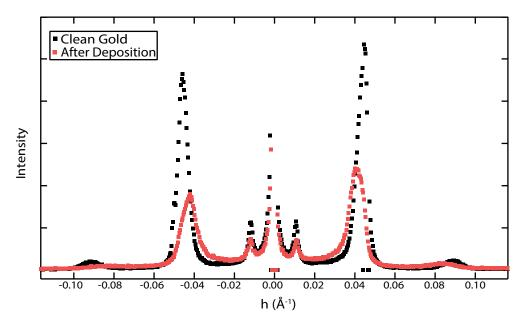
FIGURE 3.11: h scan (0.9<k<1.1; l=0.05) of the LuPc $_2$ /Au(111) sample around the ( $1\overline{1}0$ ) peak of the substrate.
