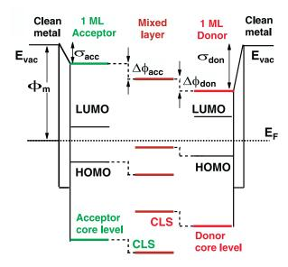
FIGURE 1.8: Schematic of the energy level alignment of the interface between a metal contact and an OSC donor/acceptor mixture. The dotted lines show the shift of the molecular levels upon vacuum level pinning. Taken from ref. [44].
