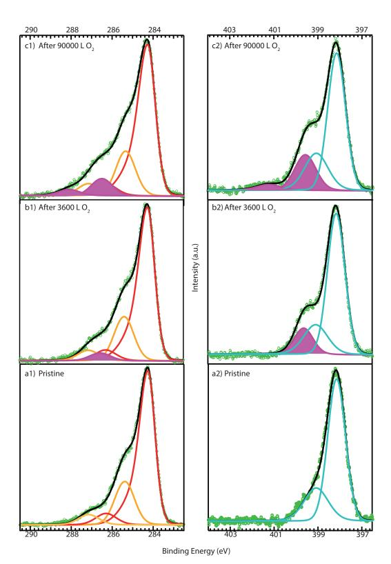
Figure 4.7: Fitting results on the C 1s (left) and N 1s (right) peak for the clean LuPc $_2$ /Au(111) film (a), after 3600 L (b) and after 90000 L (c)  $O_2$  at 88 K.
