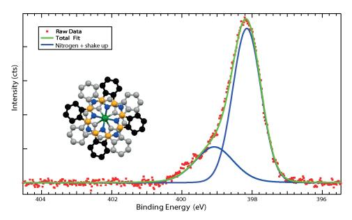
FIGURE 4.2: Resolution of the single spectral components of XPS spectrum of the N 1s peak of a LuPc<sub>2</sub> thin film ( $\sim$ 1 nm) deposited on Au(111).
