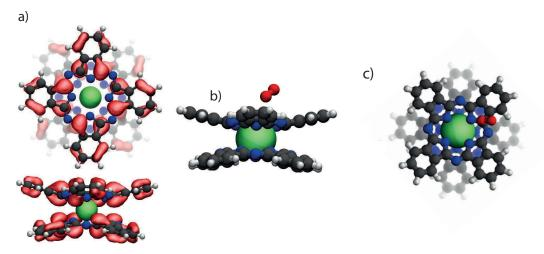
FIGURE 4.8: Molecular orbitals of  $LuPc_2$  as calculated by DFT (taken from ref. [10](a)); Geometry of oxygen absorption on isolated  $LuPc_2$  molecule as calculated by DFT seen from side (b) and top (c).
