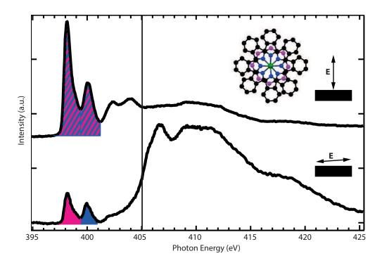
FIGURE 4.4: NEXAFS spectrum of a  $\sim$ 1 nm thick LuPc<sub>2</sub> deposited on Au(111). (top) with polarization perpendicular (90°) to the surface (out-of-plane), (bottom) with polarization parallel (4°) to the surface (in-plane). The filling represents the contributions: pyrrolic (blue) and azabridge (purple) N atoms.
