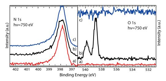
FIGURE 4.5: XPS spectra of the N 1s peak of LuPc<sub>2</sub>/Au(111) during and after exposure to water (left) and oxygen (right) in the Near Ambient Pressure regime. a)pristine LuPc<sub>2</sub> film, b) during oxgygen dose, c) after oxygen has been pumped out.
