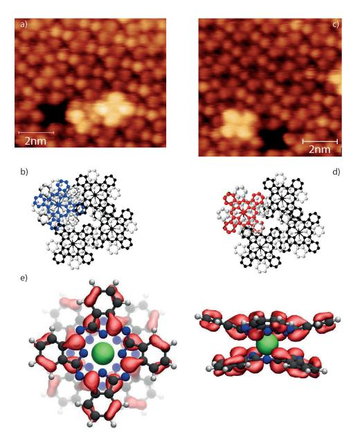
FIGURE 3.19: (a-b)STM image and molecular model of the "on top" adsorption configuration V=-2.5 V; I=300 pA; (c-d) STM image and molecular model of the "staggered" configuration V=-2.5 V; I=300 pA; (e) molecular orbitals of LuPc $_2$  as calculated by DFT in ref. [10].
