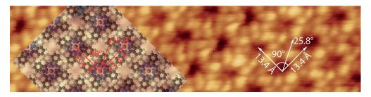
FIGURE 3.22: Calculated DFT lattice for  $LuPc_2$  monolayer adsorbed on Au(111) (left), superimposed on the measured STM image (right) V=-2.5~V; I=300~pA.
