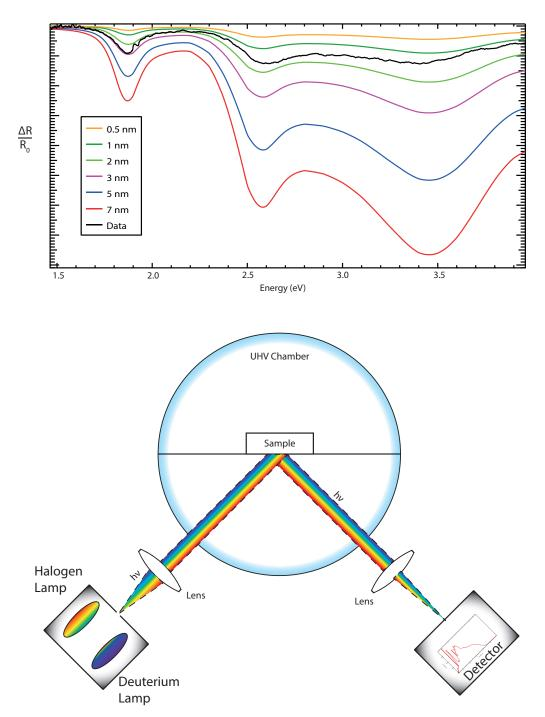
Figure 2.14: a) schema depicting the experimental setup used in this work; b) the calculated SDRS spectrum for LuPc $_2$  thin film deposited on gold, with the Data relative to a  $\sim$ 2 nm thick film obtained experimentally.
