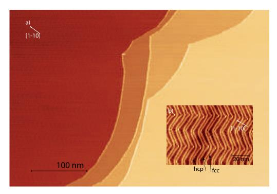
FIGURE 3.12: STM images of the Herringbone reconstruction of Au(111). Large scale a) and small smaller scale b). V=-0.3 V, I=300 pA.
