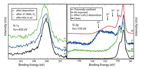
FIGURE 4.17: left: XPS spectra of the N 1s peak as deposited (a), after 27000 L  $O_2$  (b) and after air exposition. right: Si 2p spectrum of the clean sample (a), after LuPc<sub>2</sub> deposition (b), after exposition to air (c) and a thermally oxidized sample for comparison (d). References for the Silicon oxides BE are taken from ref.[41].
