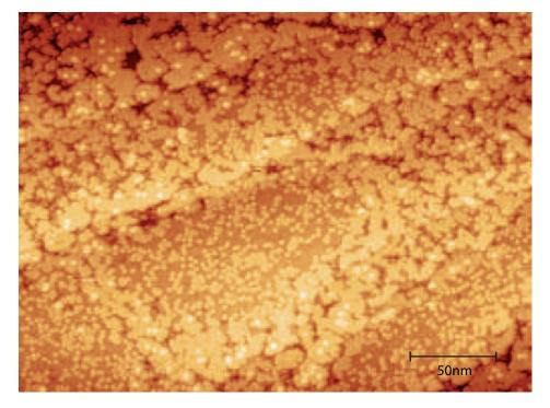
Figure 3.14: Large scale STM image of the sample after 10 minutes annealing at  $250^{\circ}$ C. V= -3 V; I=300 pA.
