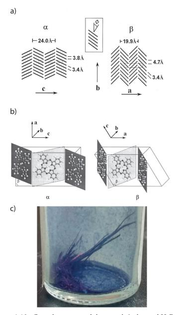
FIGURE 1.10: Crystal structure of the  $\alpha$  and  $\beta$  phase of  $H_2Pc$ . (a) Schematic depiction of the  $\alpha$  (left) and  $\beta$  (right) projected on the (100) and (001) plane respectively. (b) view of the molecular plane arrangement in the structure. c) needle like shape of crystals of CuPc. Image a) and b) taken from ref. [152].
