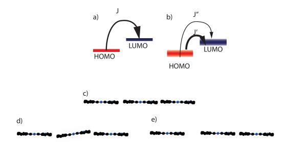
FIGURE 1.7: top:Energy level scheme for a perfectly ordered ideal system (a) showing a localized state and a real disordered system (b) showing a larger, less localized state; J is the overlap integral, the size of the arrow is proportional to the integral value. Bottom: perfectly ordered ideal system c), examples of possible off diagonal disorder: rotation d) or displacement e) of a molecule in the lattice.
