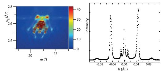
FIGURE 3.7: Inplane mesh (l=0.05) of the (110) peaks of the clean Au(111) substrate (left) and cut along one of the diagonal of the reciprocal space comprehending the herringbone reconstruction (right). The cut has been projected on the **h** vector of the reciprocal lattice for ease of representation.
