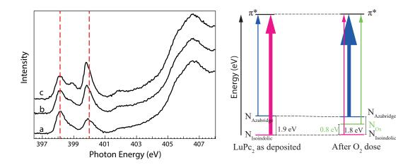
FIGURE 4.10: Zoom on the  $\pi^*$  transitions for the pristine LuPc<sub>2</sub> molecule a), after a 3600 L oxygen dose b) and after a 90000 L dose c)(left); the energy levels involved in the  $\pi^*$  transitions, the arrow size is proportional to the transition intensity (right).
