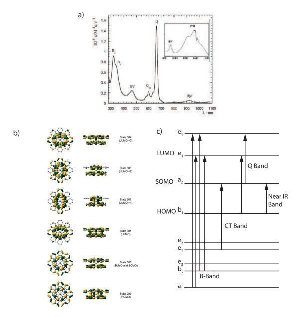
FIGURE 1.13: Optical absorption spectra of the molecule in dichlorometane (a); Frontier orbitals for  $LuPc_2$  as calculated by DFT (b); spatial localization of the frontier orbitals(c). (a) taken from ref. [12]; (b) adapted from ref. [120] and (c) from ref. [101].
