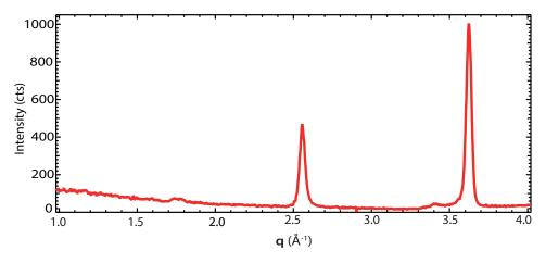
FIGURE 3.5:  $\theta/2\theta$  scan on a 200 nm thick LuPc<sub>2</sub> thin film on Au(111).
