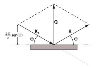
FIGURE 2.17: Geometry of the scattering vector construction.
