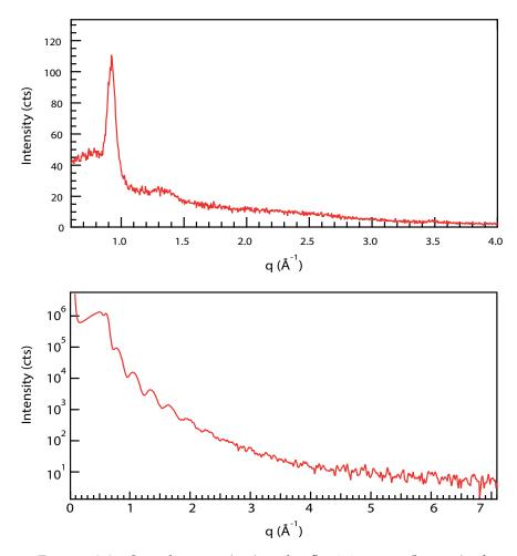
Figure 3.2: Specular scan (top) and reflectivity scan (bottom) of  $LuPc_2$  deposited on H terminated Si(100).
