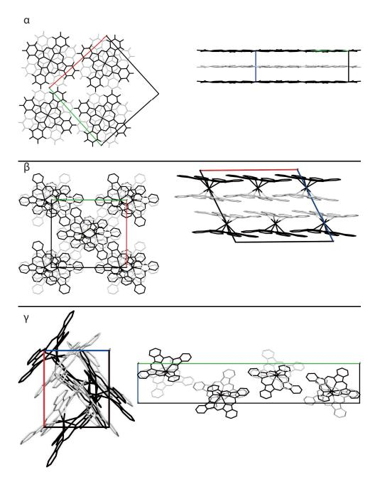
FIGURE 3.1: top:  $\alpha$  phase from CuPc as taken from ref. [133], the molecules belonging to the lower planes are coloured in lighter colour; centre: the  $\beta$  structure from NdPc<sub>2</sub> taken from ref. [34]; bottom: the  $\gamma$  structure from LuPc<sub>2</sub> taken from ref. [98]. The atoms belonging to the lower plateau of double-decker phthalocyanine and the second plane in the structure of single decker phthalocyanine are coloured in lighter colours for clarity.
