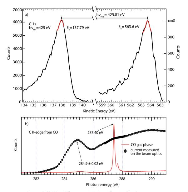
FIGURE 2.13: Two different methods for calibrating the photon energy in NEXAFS spectra: a) Carbon 1s spectrum measured using the first (left) and second (right) diffraction order of the monochromator. The peaks have been fitted with a Gaussian curve. b) internal standard using the impurities on the monochromator. Image b) courtesy of L. Floreano.
