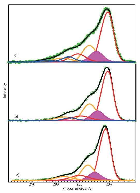
FIGURE A.4: C 1s spectra of a LuPc $_2$   $\pm 1$  nm thick sample deposited on Au(111) after 2h irradiation (a), after 5h irradiation (b) and after 10h irradiation (c).
