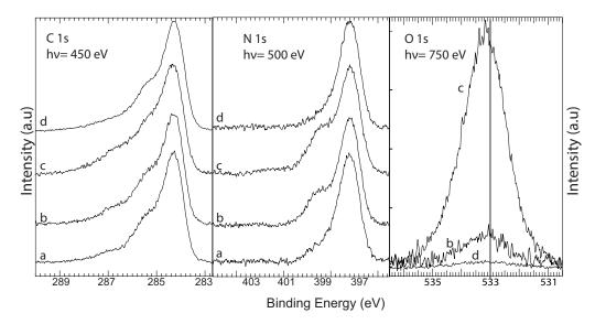
FIGURE 4.6: XPS spectra of  $LuPc_2/Au(111)$ . C 1s (left) and N 1s (centre) and O 1s (right) before (a) after 3600 L (b) after 90000 L (c) of oxygen at 88 K, and after heating up (d) at room temperature.
