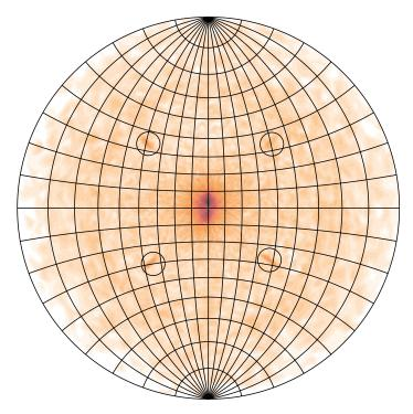
FIGURE 3.3: Pole figure around the (040) peak of LuPc<sub>2</sub> on H terminated Si(100).
