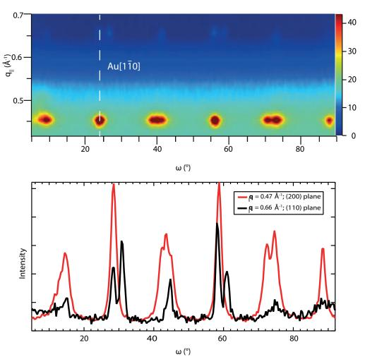
FIGURE 3.9: (Top)In-plane mesh (l=0.05) of the LuPc $_2$ /Au(111) sample after heating to 285°C . The position of the 110 peak of gold is at 84.0 $\pm$ 0.3°, marked by the vertical line. (bottom) cut along two lines to evidence the alternating pattern of the peaks.
